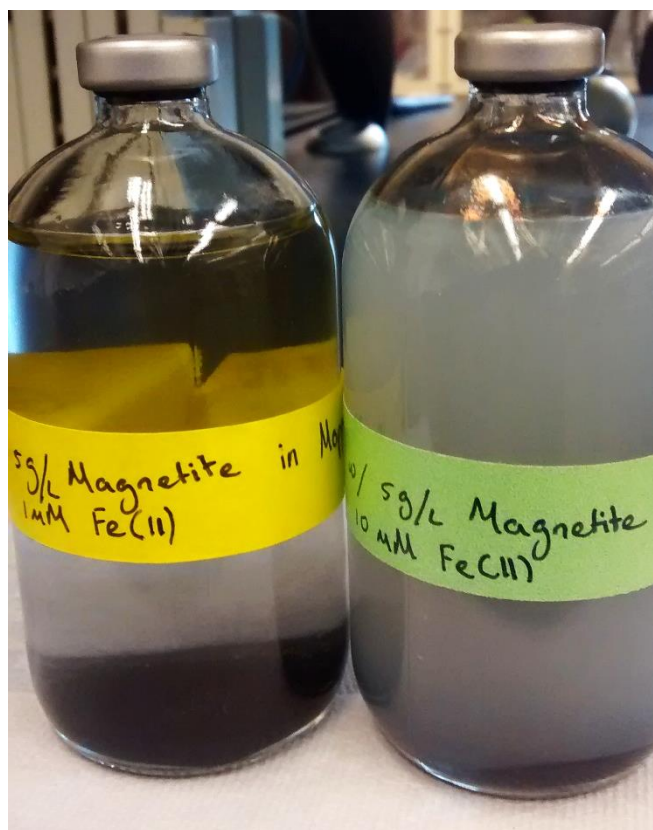
Figure S1. Photographs of reactors containing 5 g/L magnetite reacted with low Fe(II) (~1 mM, left) and high Fe(II) (~10 mM, right). The solids on the right contain white \text{Fe}(\text{OH})_2(\text{s}) . Conditions: 10 mM MOPS buffer at pH 8.0, and 50 \mu\text{M} TCE.
