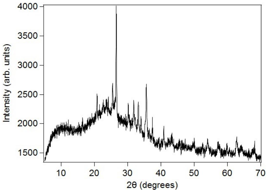
**Figure S1.** A representative XRD diffractogram taken from 5° - 70°. The XRD is an untreated Clifty sample and shows the higher angles (above 45°) that were not included in Fig. 1. At these higher angles, the intensity decreases making it difficult to differentiate between the components when labelling. The large bumps at 10° and 25° are likely due to amorphous components of the fly ash samples.
