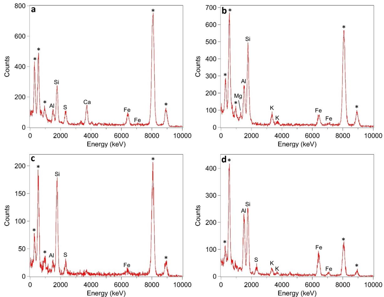
**Figure S3.** EDS spectra of the particles shown in Figure 3 of untreated Class F (a and b) and acid-treated Class F (c and d). The labels from Figure 3 correspond to the same letter in this figure. The elements are labeled by symbol in each spectrum. EDS peaks from background signals of C, O, and Cu are denoted by \*.
