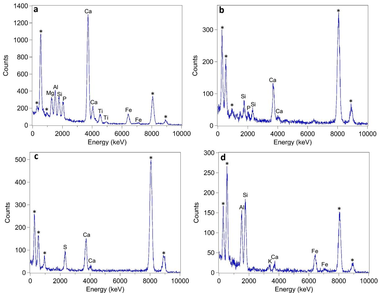
**Figure S2.** EDS spectra of the particles shown in Figure 2 of a) spherical, untreated Class C, b) irregular, untreated Class C, c) acid-treated Class C, and d) acid-treated Class C/F. The labels from Figure 2 correspond to the same letter in this figure. The elements are labeled by symbol in each spectrum. EDS peaks from background signals of C, O, and Cu are denoted by \*.
