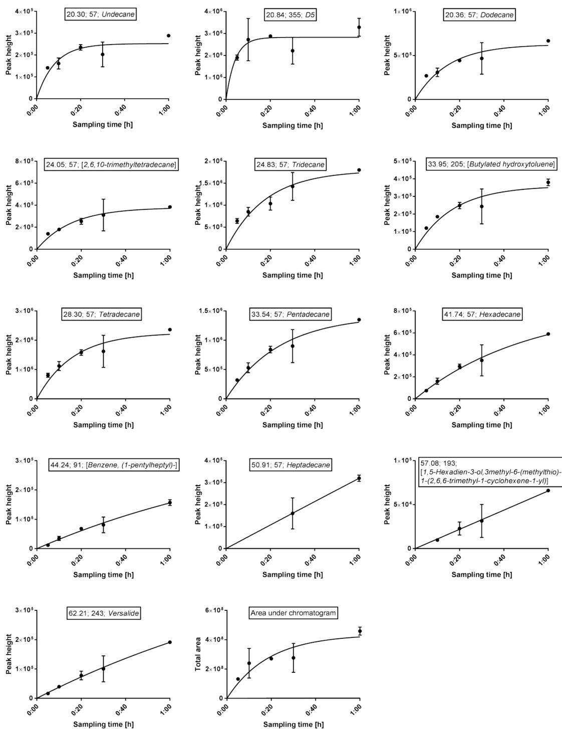
Figure ESI1: Base peak heights of selected molecular features at 5, 10, 20, 30 and 60 mins of sampling time.  $n=2$ . Curves are modeled by  $Y = \text{Plateau} * e^{-K*t}$ , where  $K$  is the rate constant, and  $t$  the time in minutes.
