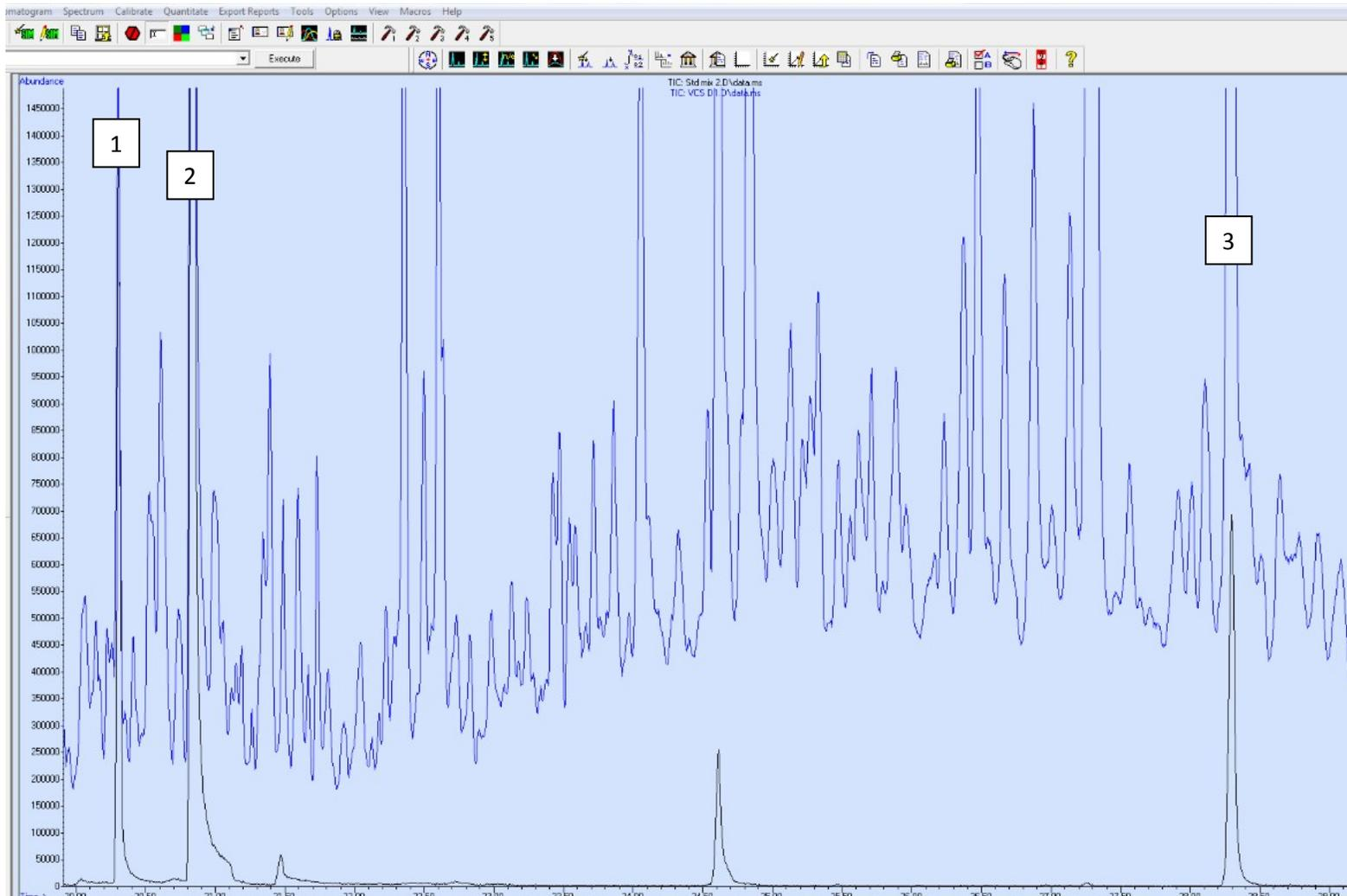
Figure ESI3: Chromatographic data supporting identification of undecane (1), D5 (2), and tetradecane (3). Retention time match in full scan run of digested sludge sample (blue) and composed standard mix consisting of 0.01% undecane, D5 and tetradecane in Miglyol oil (black). The corresponding mass spectra are shown in Table ESI2.
