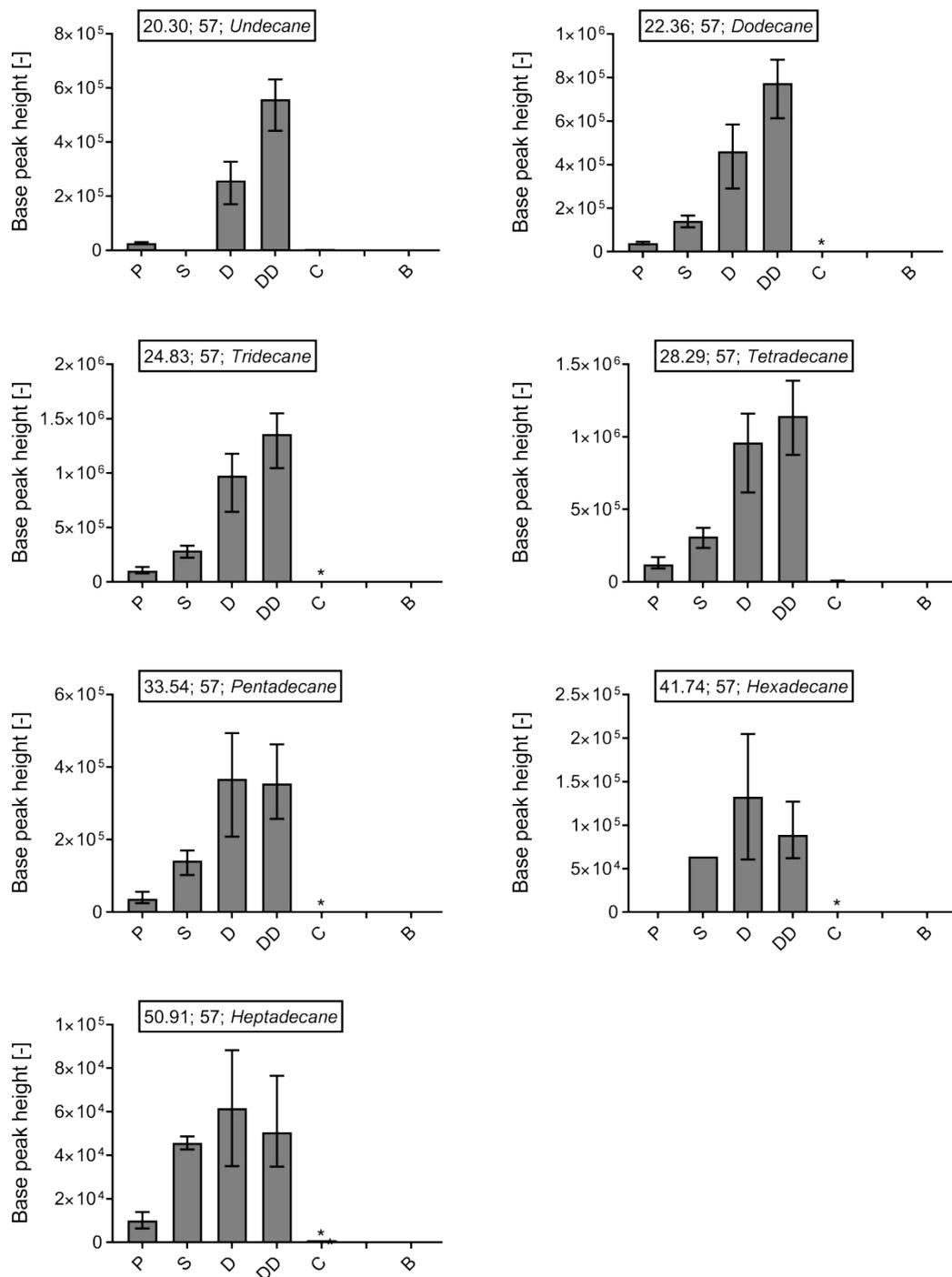
Figure ESI5: Base peak heights from MassHunter deconvolution on digested sludge for alkanes included in Fig. 3. Values below data processing threshold limit (peak height < 5000) were manually checked and marked with a \* if present in the chromatogram and data manually extracted in ChemStation.
