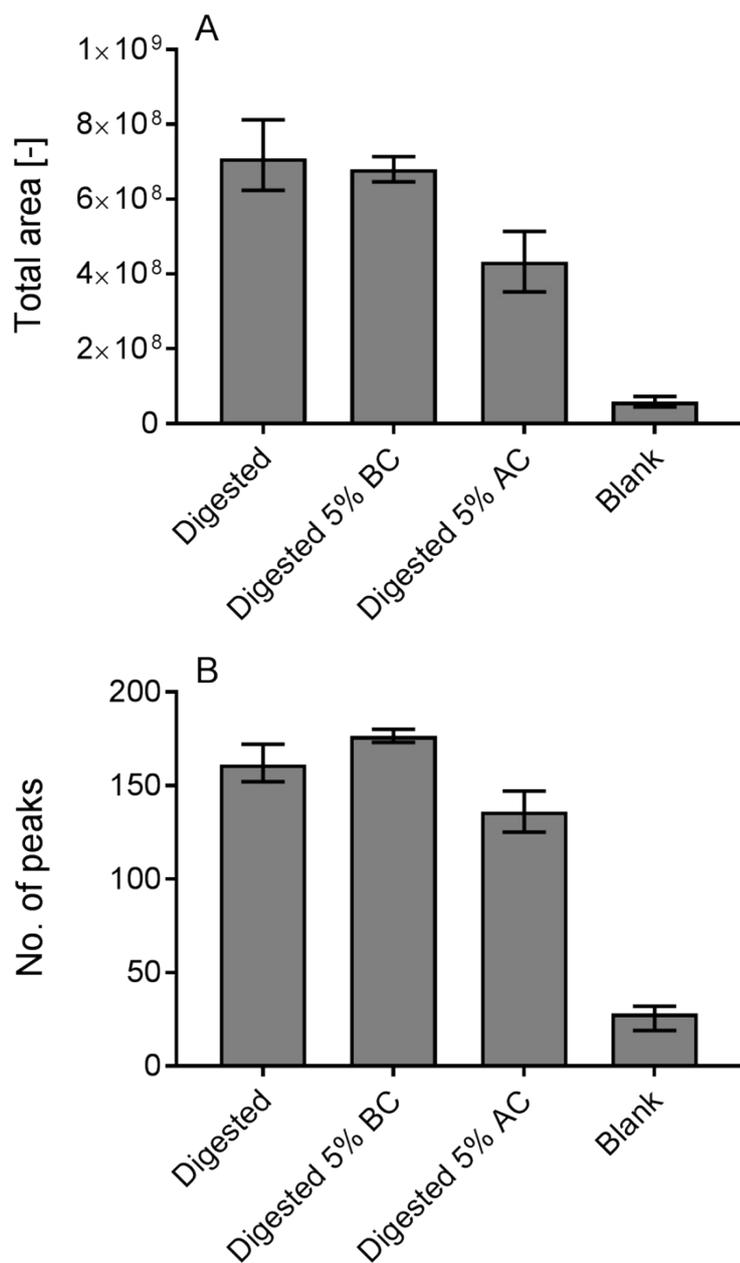
Figure ESI6: Sum of peak areas (A) and number of peaks (B) of molecular features extracted by MassHunter from 15 to 60 min retention time, measured in non-treated digested sludge, digested sludge with 5% amendment of activated carbon (AC) and digested sludge with 5% amendment of biochar (BC) and in a blank sample.
