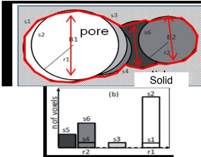
Figure S2: Schematic view of the I-Morph operator to obtain the granulometric volume distribution of the void phase
