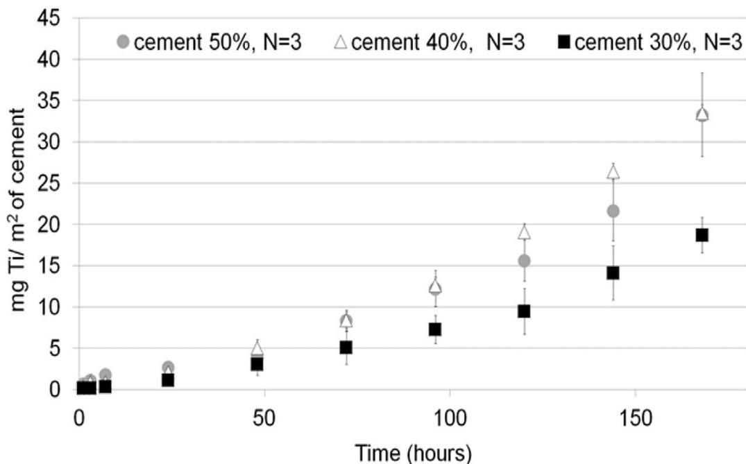
**Figure S4: Total amount of particulate Ti released during leaching of hardened cement 30, 40 and 50% over a time course. Released amounts are normalized by the cement external surface (extracted from<sup>1</sup>)**
