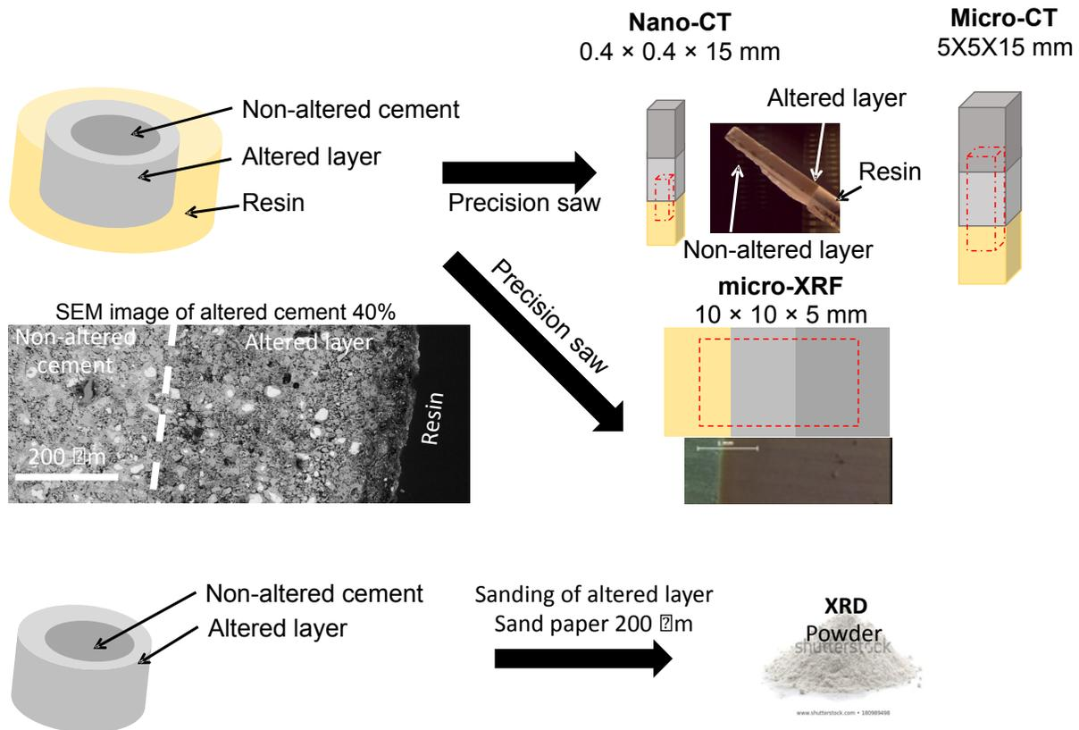
**Figure S1: Schematic view of altered sample preparation for X-ray analysis ( XRD, micro-XRF, Nano-CT and Micro-CT)**
