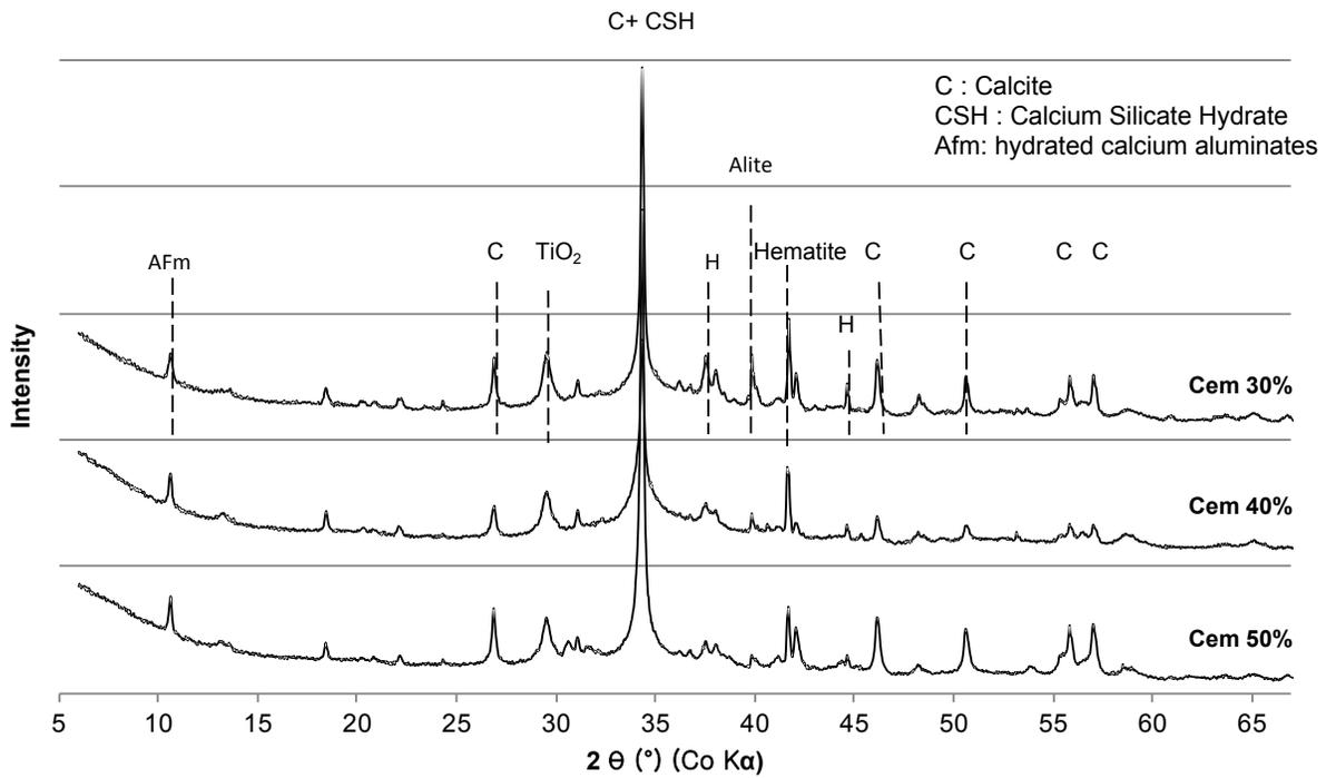
**Figure S3: X-ray diffraction (XRD) patterns of cement 30%, cement 40% and cement 50% of the first 100 microns of the altered layer. Hematite is coming from the sand paper used to remove the very altered layer of cement pellets.**
