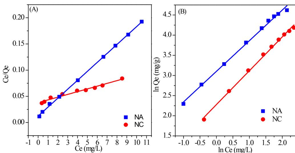
**Figure S2.** Langmuir (A) and Freundlich (B) kinetic models of U(VI) on NA and NC
