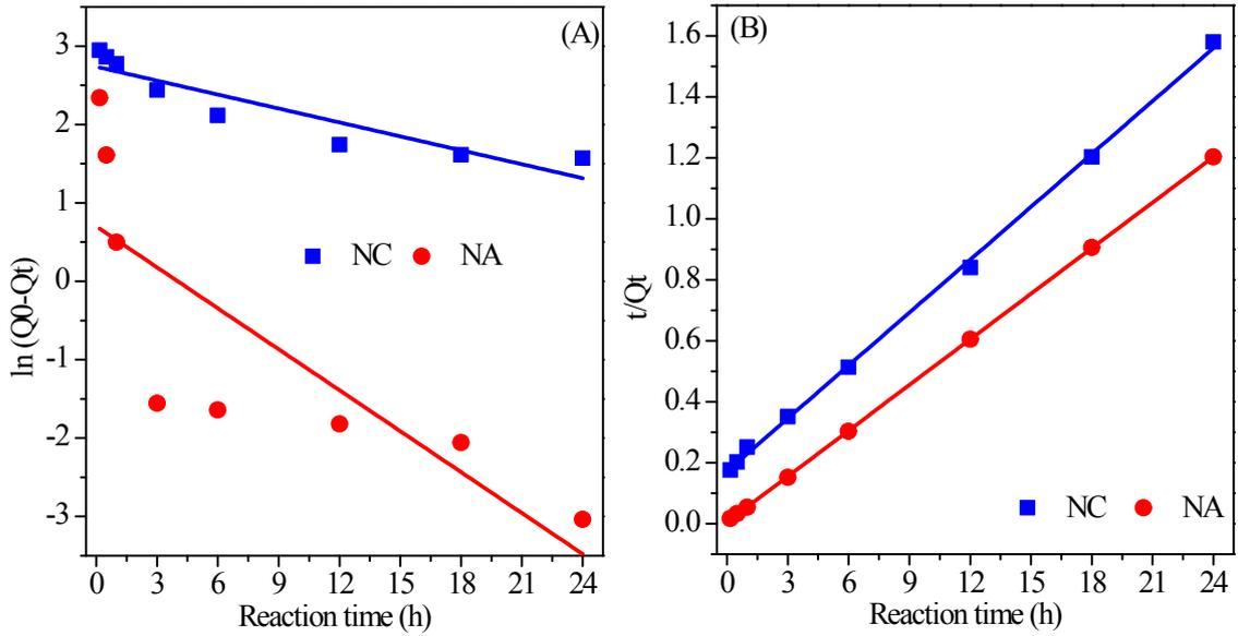
**Figure S1.** Pseudo-first-order (A) and pseudo-second-order (B) kinetic models of U(VI) on NA and NC, pH 4.0,  $I = 0.01$  mol/L,  $m/v = 0.5$  g/L,  $T = 293$  K.
