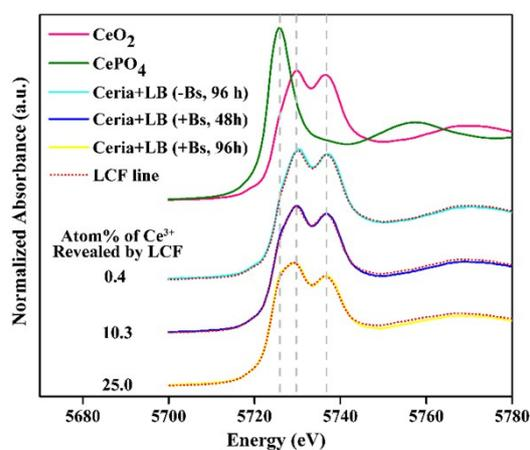
**Fig. S3.** Ce LIII-edge XANES spectra. XANES spectra of reference standards: bulk  $\text{CeO}_2$  and  $\text{CePO}_4$ ; XANES spectra of samples: 100  $\mu\text{g/mL}$  rod-ceria incubated in the LB medium with or without *B. subtilis* for 48 or 96 hours; the LCF line and the fitting result.
