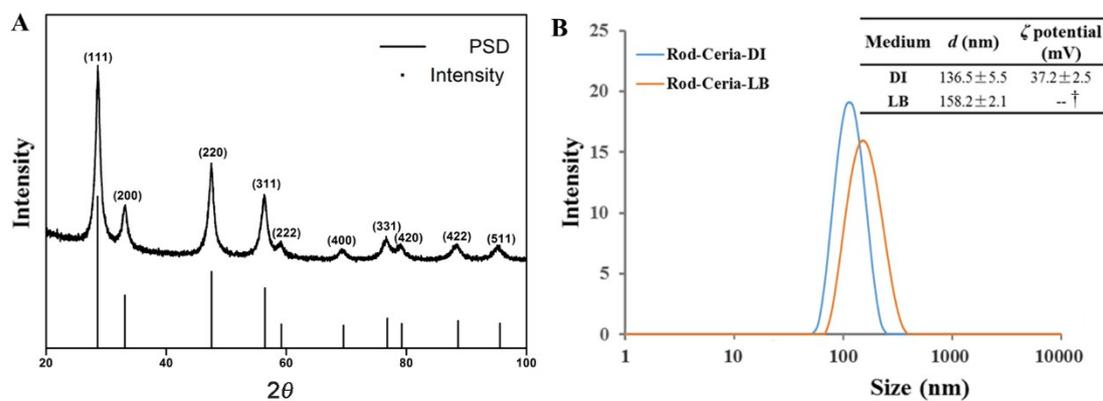
**Fig. S1.** The physicochemical properties of rod-ceria. A) The XRD patterns of rod-ceria (JCPDS card no. 34-0394). B) Size distribution and zeta potential of rod-ceria in the deionized water (DI) and LB medium were measured by dynamic light scattering assay; †: the zeta potential of rod-ceria in LB culture medium could not be determined due to the high sample conductivity.
