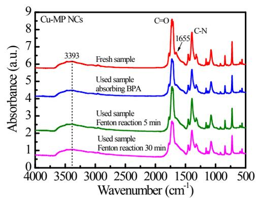
**Figure S7.** FTIR spectra of the Cu-MP NCs samples after absorbing BPA and after Fenton-like reaction with BPA.
