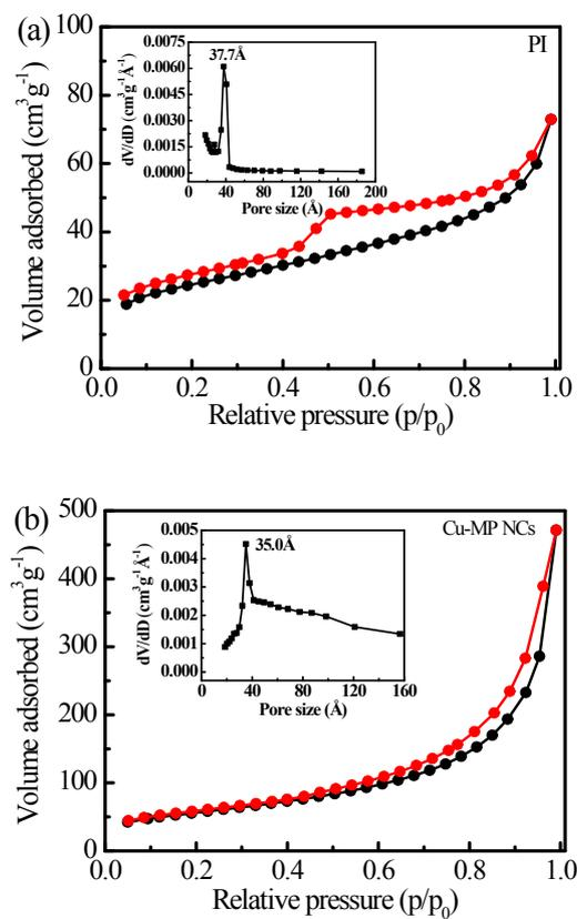
**Figure S2.** N<sub>2</sub> adsorption-desorption isotherms and BJH pore size distribution (inset) of (a) PI and (b) Cu-MP NCs.
