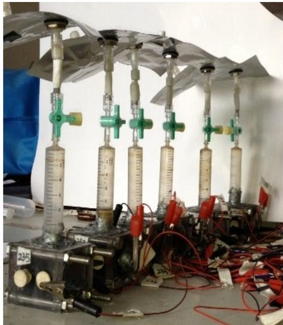
Figure S1 Experimental single chamber microbial electrolysis cells
