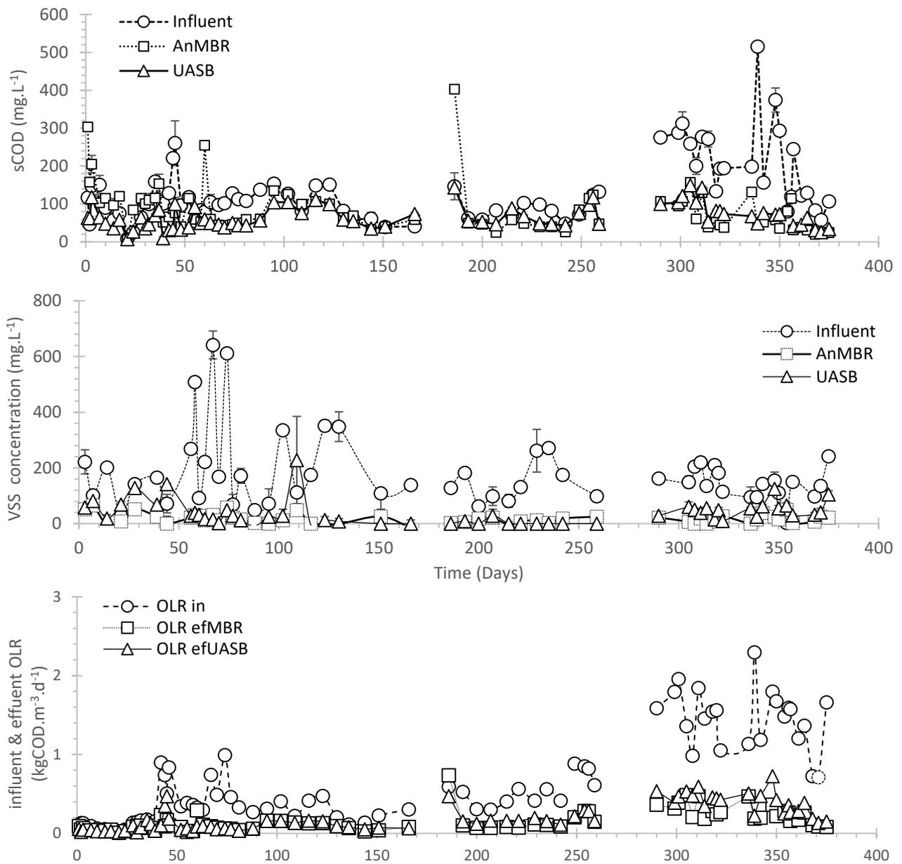
Figure S2 – Concentration(s) of (top to bottom): soluble COD (sCOD); volatile suspended solids (VSS); in the influent and effluent for both the AnMBR and UASB; influent and effluent OLR for the two systems. Error bars stands for standard error (n=2).
