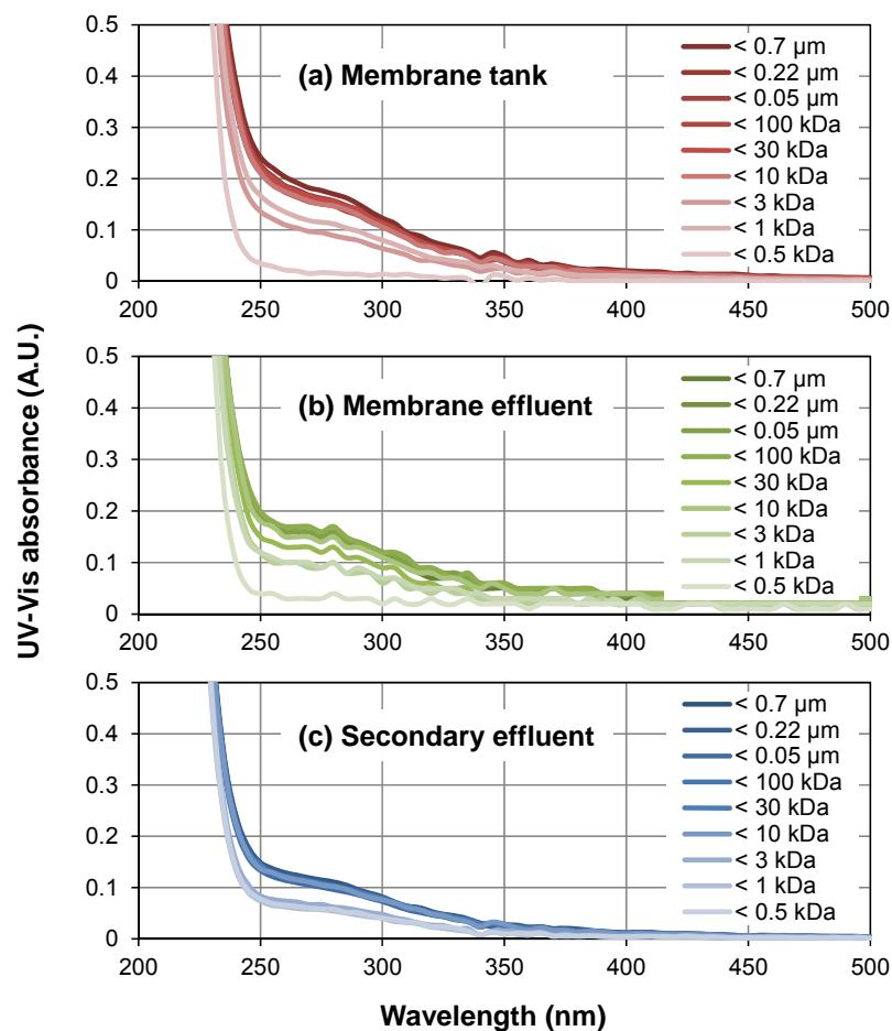
**Fig. S2.** UV-Vis spectra of DOM with different molecular weight/size levels from (a) membrane tank, (b) membrane effluent, and (c) oxidation ditch secondary effluent.
