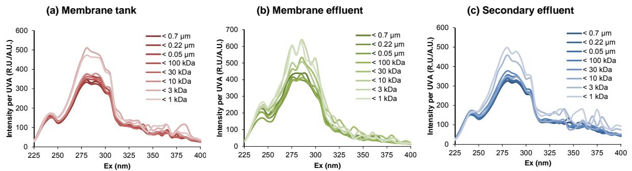
**Fig. S4.** Fluorescence excitation spectra in terms of fluorescence intensity (R.U.) per excitation UV absorbance (A.U.).
