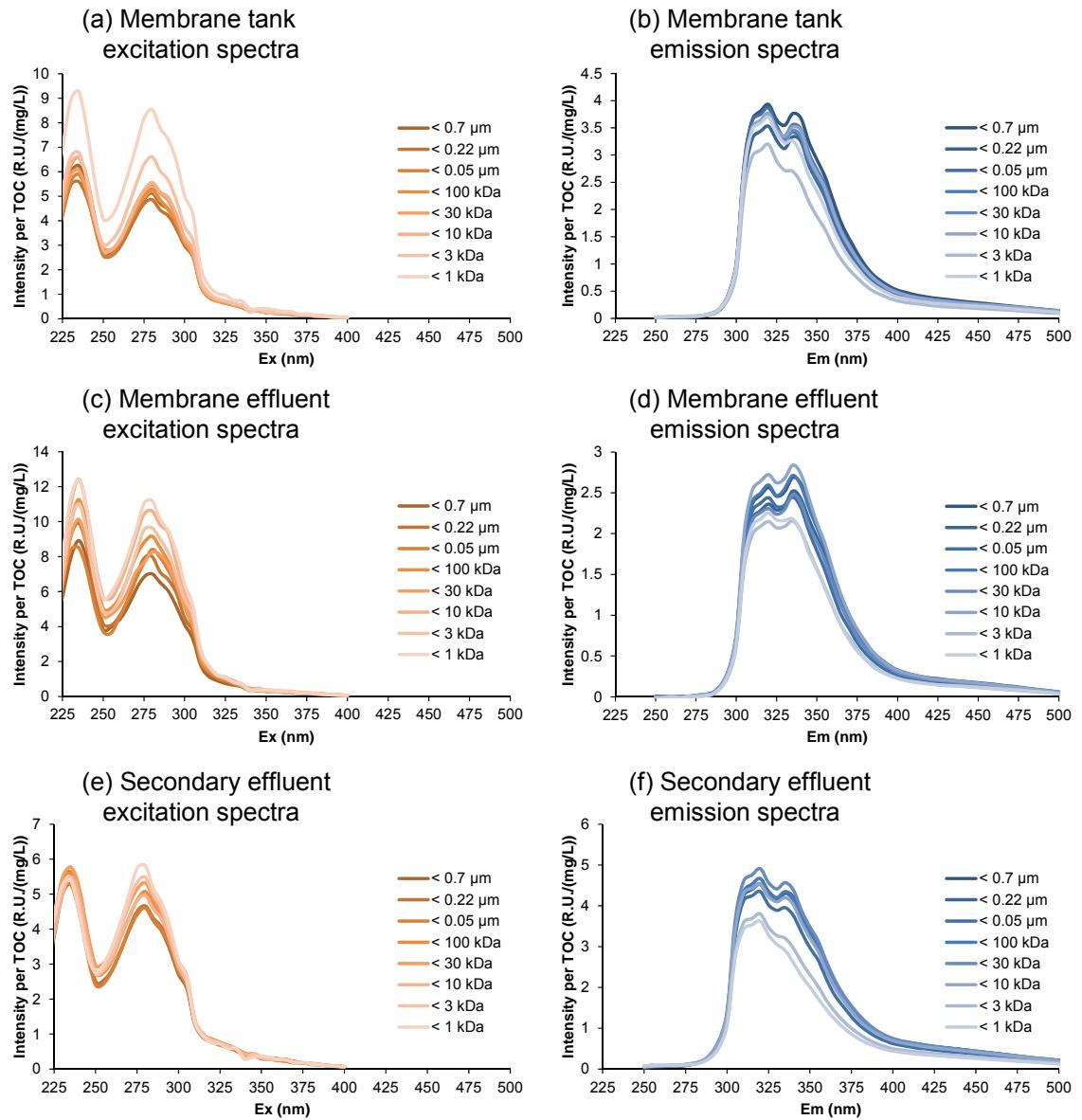
**Fig. S3.** Fluorescence excitation spectra and emission spectra of the DOM fractions.
