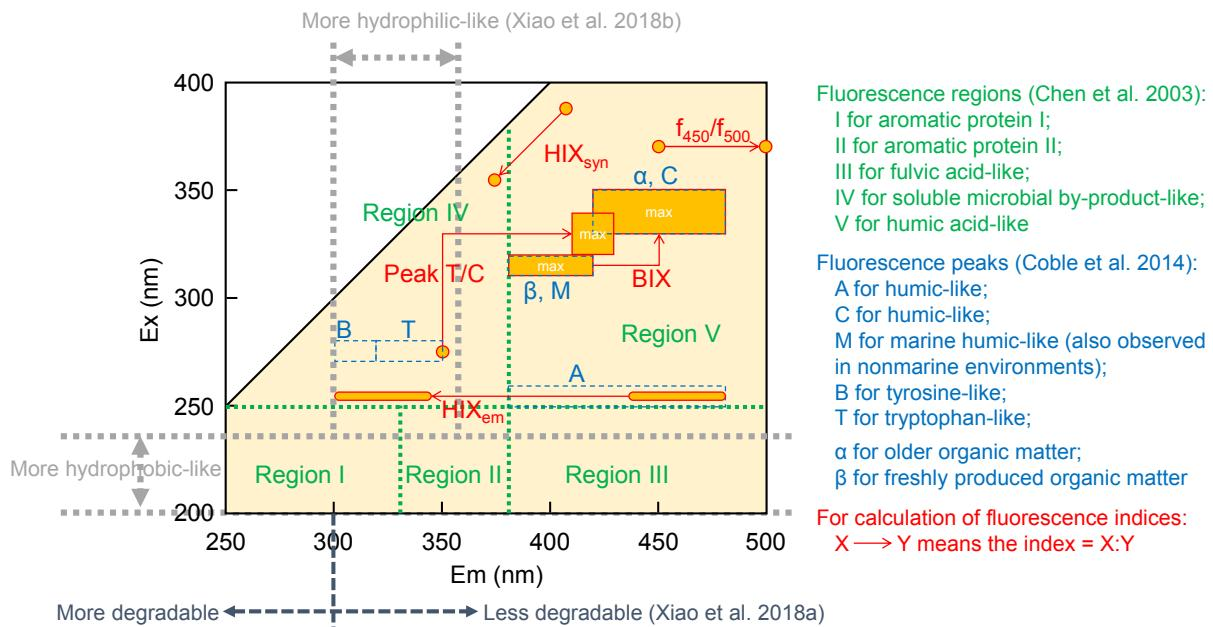
**Fig. S1.** Illustration of typical fluorescence regions, fluorescence peaks and fluorescence indices, according to the references of:
