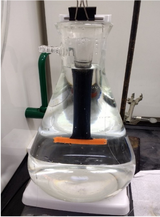
Figure S2: Brine Removal from Aq-SNR dispersion. (A) Aq-SNR is added in the form of dialyte and MilliQ is added as dialyzate. The dialyzate was replaced after every 2 h and the conductivity of dialyzate was checked as a function of the number of iterations. This confirms maximal removal of brine ( <1 \mu\text{S}/\text{cm} )
