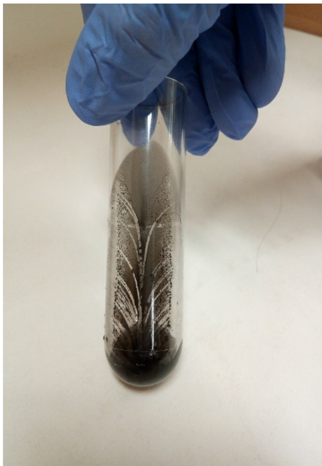
Figure S1: After centrifugation at 100,000 RCF (1 h), the reaction mixture deposits at the walls of the polycarbonate tubes
