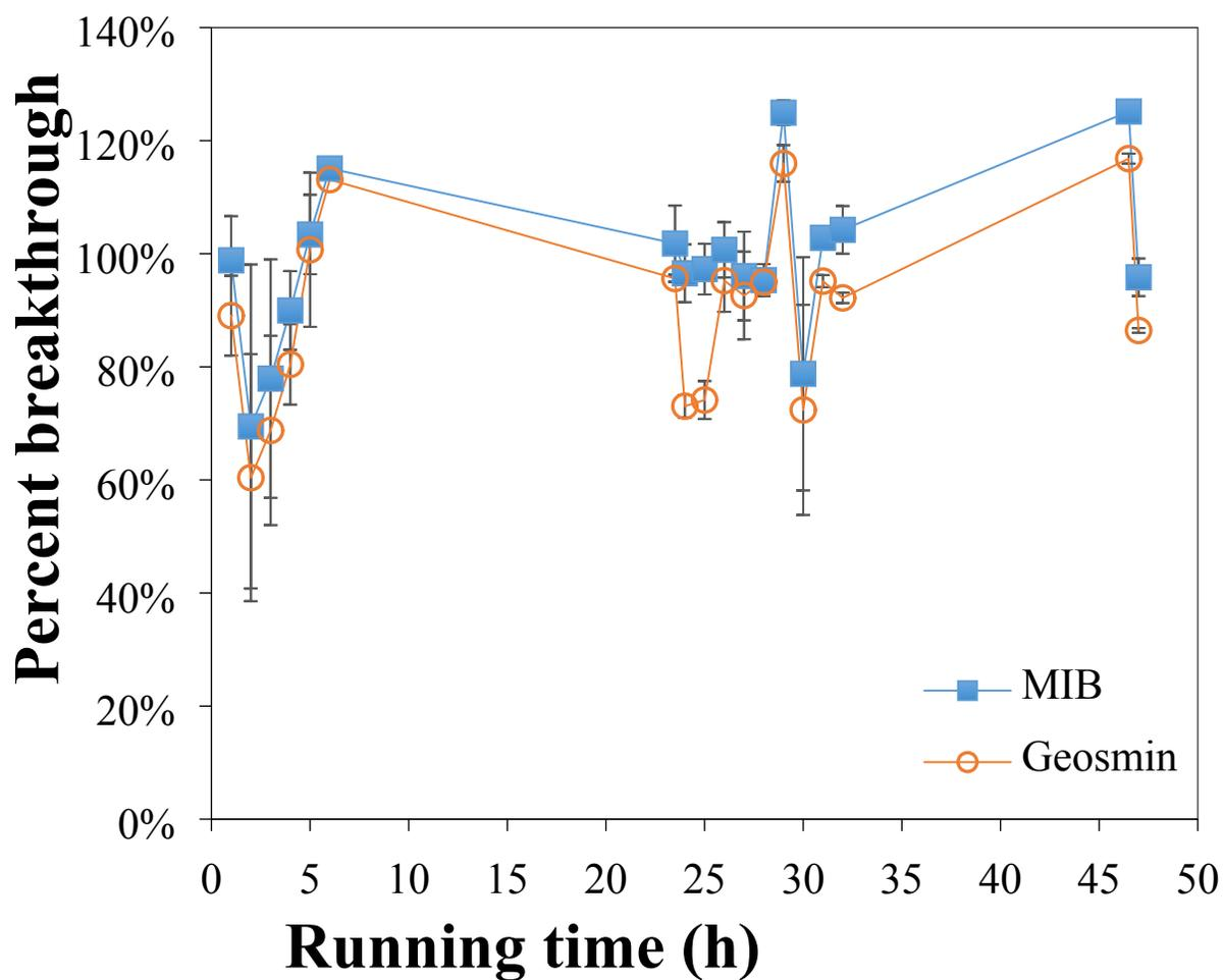
**Figure S3.** Breakthrough of MIB and geosmin from an empty pilot-scale column (error bars represent max/min values of two replicate samples from one column)
