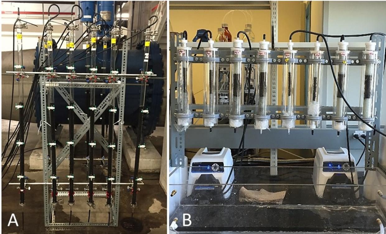
**Figure S1.** a) pilot-scale column test onsite and b) minicolumn test in the lab
