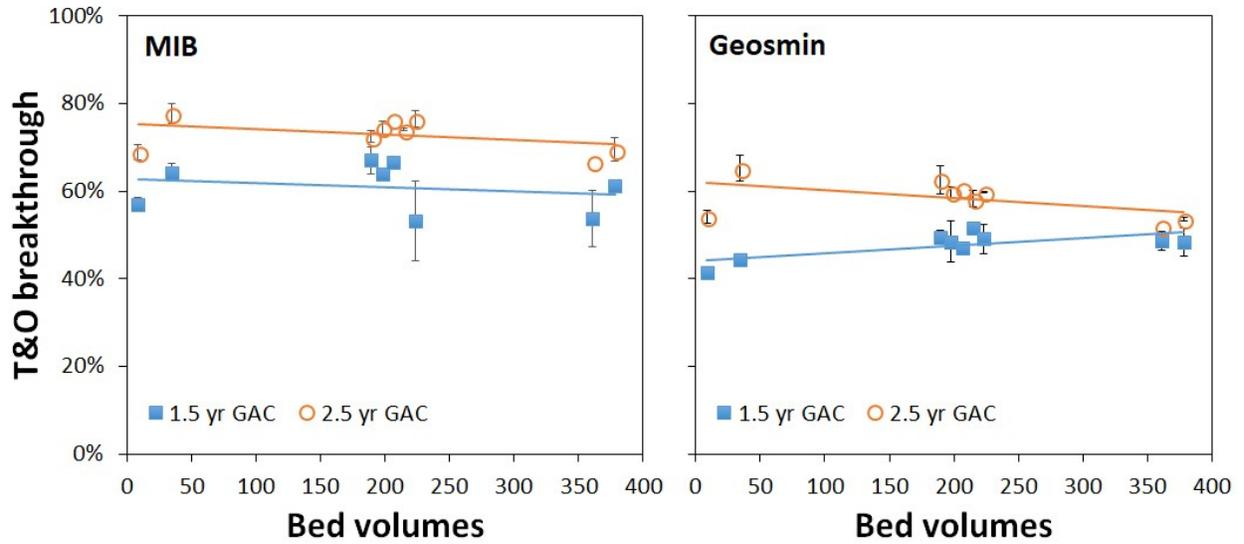
**Figure S5.** Breakthrough of MIB and geosmin vs. bed volume from the minicolumn test using pre-loaded GAC from Plant C. EBCT was 6.3 min. Column ID: 2.5 cm.
