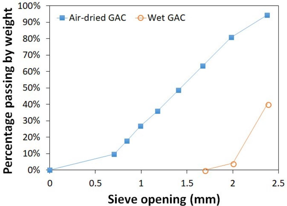
**Figure S4.** An example of particle size distributions of wet and air-dried GAC samples from Plant B
