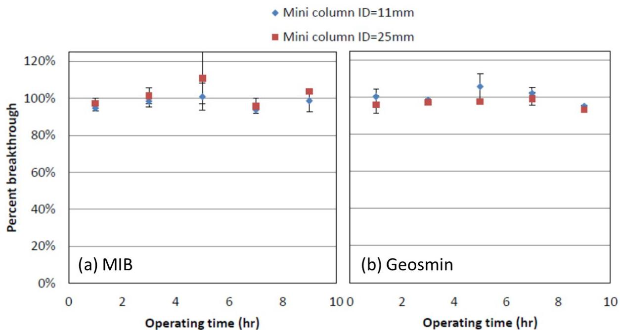
**Figure S2.** Breakthrough of a) MIB and b) geosmin over 8 hours through a blank minicolumn system packed with glass beads (error bars represent the max/min values of samples from duplicate columns)
