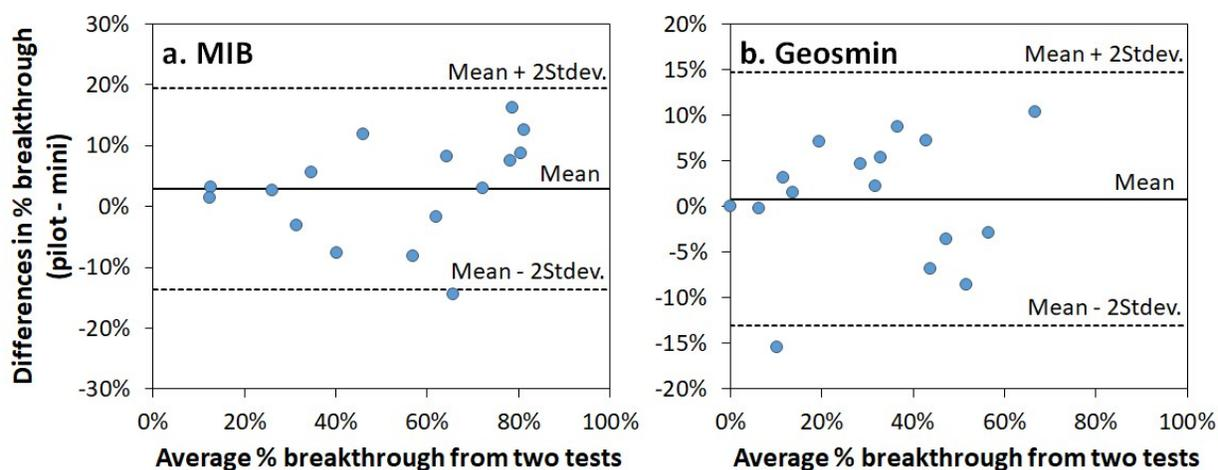
**Figure S6.** The differences between the breakthrough results of the pilot-scale column test and the minicolumn test plotted against the average breakthrough results from the two tests
