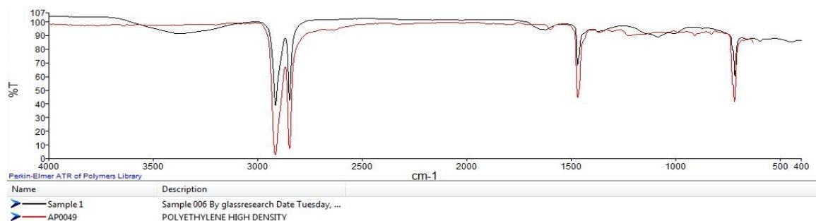
**Fig. S2** FTIR spectra for the polyethylene particles extracted from the personal care product (black line) compared to high density polyethylene (red line). The resulting spectrum for the particles had the greatest similarity with the polyethylene standard in the Perkin Elmer spectral library.
