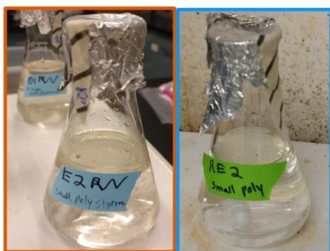
**Fig. S1** Batch reactors with either Raritan River water or wastewater influent spiked with microparticles were continuously stirred, as described Methods, to simulate the shear expected for turbulent open channel flow.
