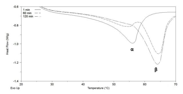
Appendix 2. Melting profiles of MG-oil mixture measured during a stop-and-return experiment at 20°C (after cooling from 80°C to 20°C at a rate of 10°C/min). The isothermal crystallization was interrupted after 1 (solid line), 180 (dashed line), or 300 (dash dot line) minutes after which the sample was heated to 80°C at a rate of 20°C/min.
