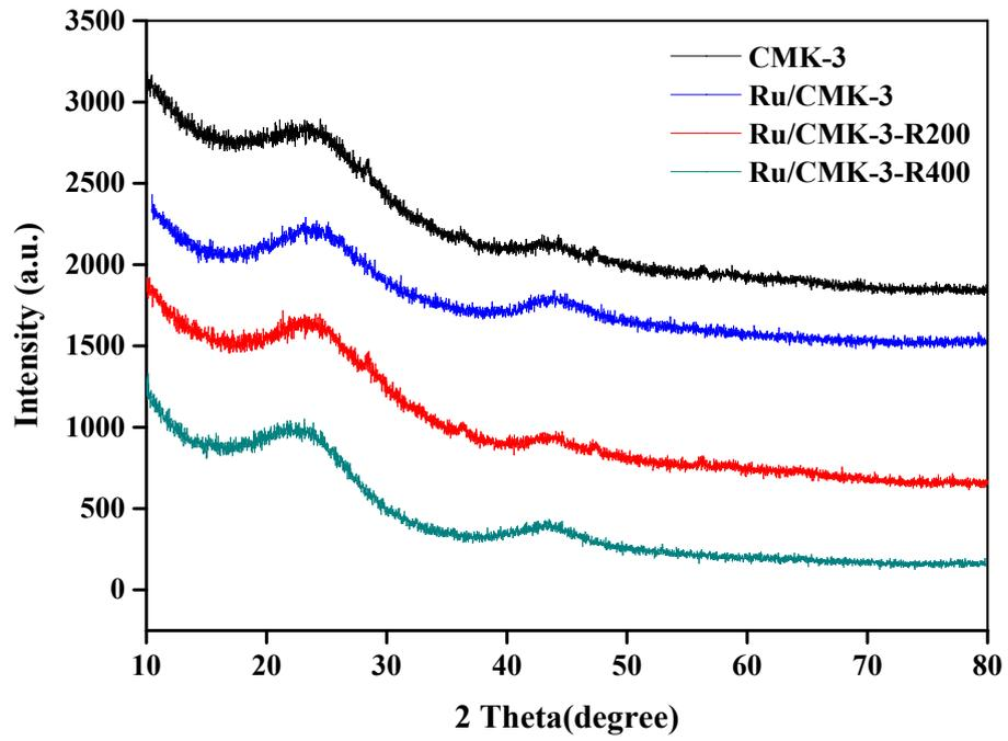
**Figure S1:** XRD patterns of CMK-3, Ru/CMK-3, Ru/CMK-3-R200 and Ru/CMK-3-R400.
