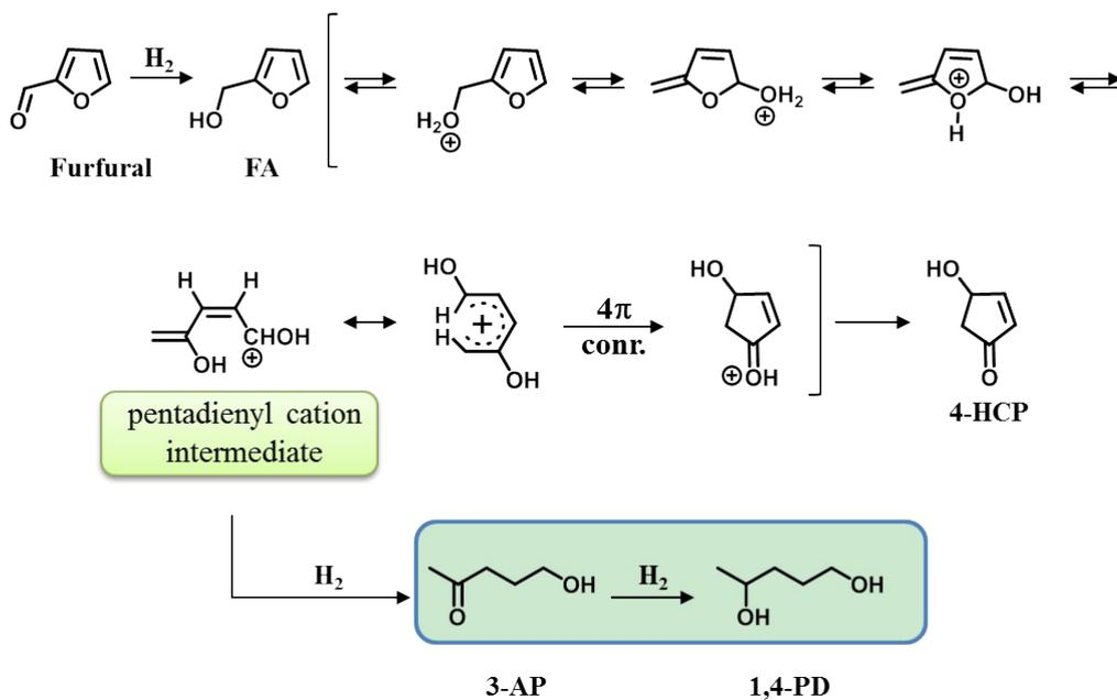
**Figure S9:** Proposed mechanism for 3-AP and 1,4-PD synthesis through a cascade sequence that terminates with the hydrogenation of a pentadienyl cation intermediate.
