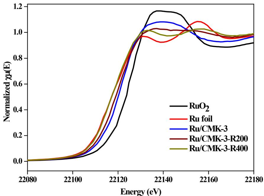
**Figure S4:** In situ XANES spectra of Ru/CMK-3-unred, Ru/CMK-3-R200 and Ru/CMK-3-R400 compared with RuO<sub>2</sub> and Ru foil.
