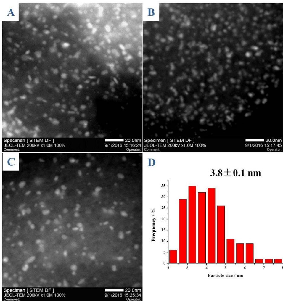
**Figure S3:** Typical HAADF-STEM images of Ru/CMK-3-R400 (A-C) and the corresponding size distribution (D).
