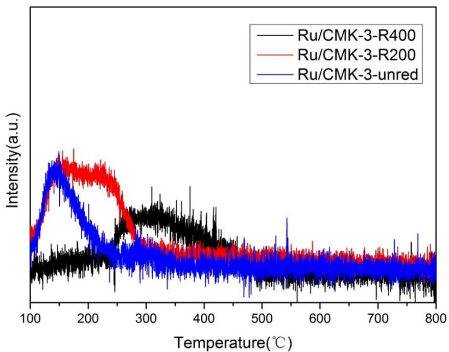
**Figure S5:** NH<sub>3</sub>-TPD profiles of Ru/CMK-3 catalyst
