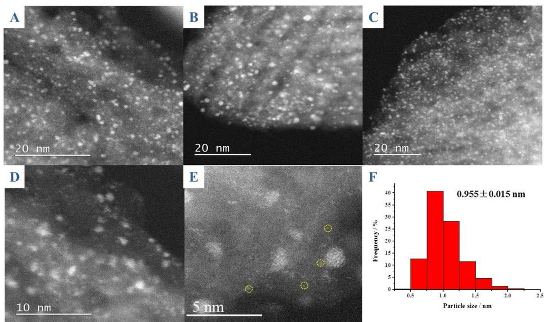
**Figure S2:** HAADF-STEM images of Ru/CMK-3-R200 (A-E) and the corresponding size distribution (F).
