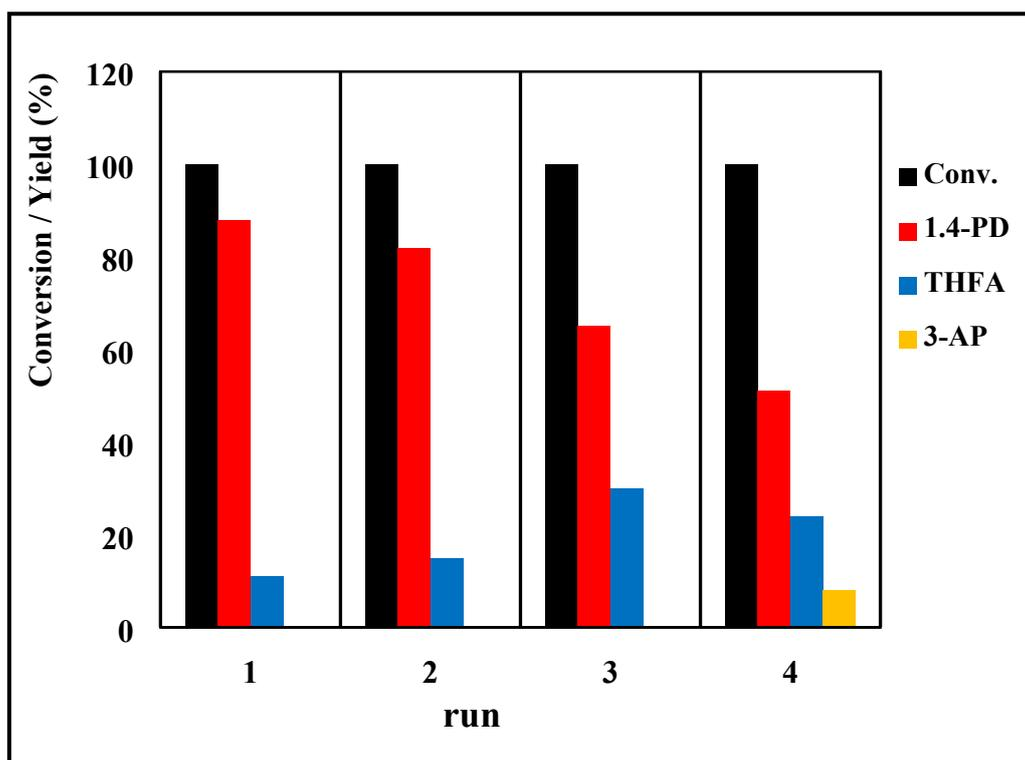
**Figure S7:** Recycling test of Ru/CMK3-R200 catalyst. Reaction conditions: 2 wt% furfural in H<sub>2</sub>O, 5 mL H<sub>2</sub>O, 20h and a metal/substrate ratio of 0.57 mol%.
