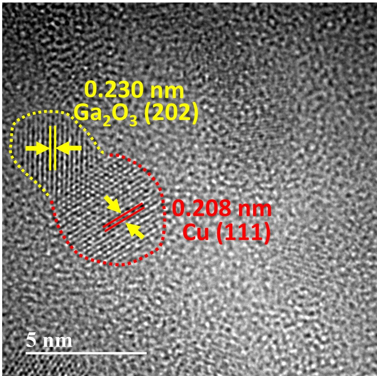
**Fig. S4** High-magnification HR-TEM image of the 5C-2G catalyst. Yellow and red lines indicate the (202) and (111) lattice plane corresponding to  $\text{Ga}_2\text{O}_3$  and  $\text{Cu}$ , respectively.
