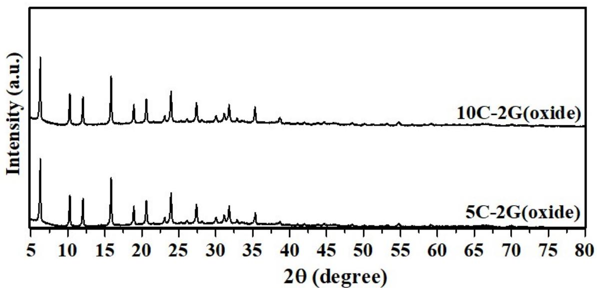
**Fig. S2** XRD patterns of the Ga-doped Cu/HNZY (oxide form).
