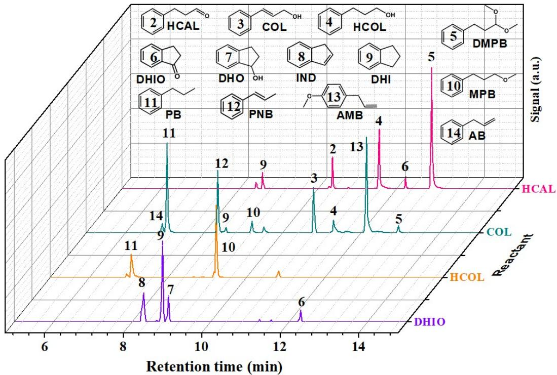
**Fig. S9** GC-TOF/MS chromatograms of the liquid products obtained from the selective hydrogenation/hydrodeoxygénération of hydrocinnamaldehyde (HCAL, 2), cinnamyl alcohol (COL, 3), hydrocinnamyl alcohol (HCOL, 4) and 2,3-dihydroindanone (DHIO, 6) over the 10C–2G catalyst. Reaction conditions: 1 g feed, 35 ml MeOH, 0.25g catalyst, 1 h, 180 °C, and an initial H<sub>2</sub> pressure of 1 MPa.
