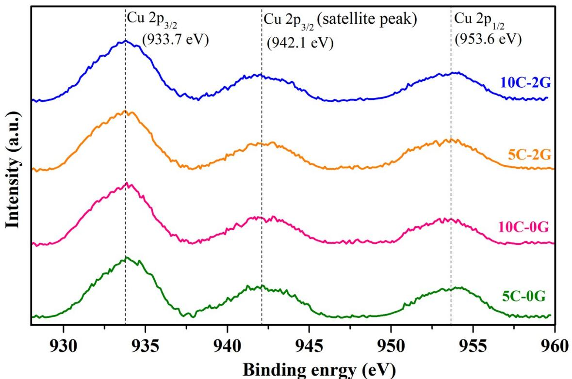
**Fig. S3** XPS core-level spectra of the Cu 2p state of Cu-based catalysts (oxide form).
