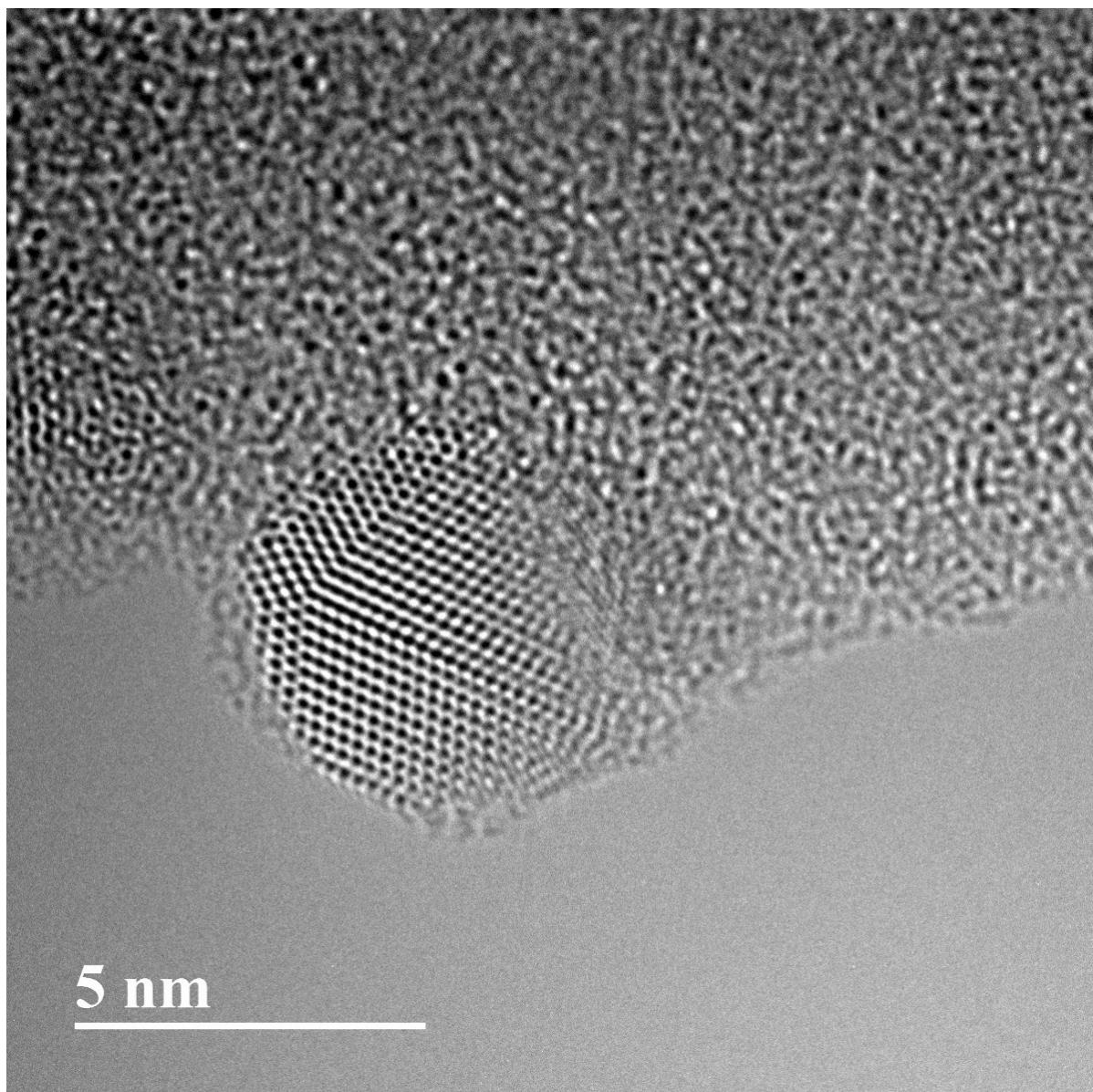
**Fig. S5** High-magnification HRTEM image of the 10C–2G catalyst.
