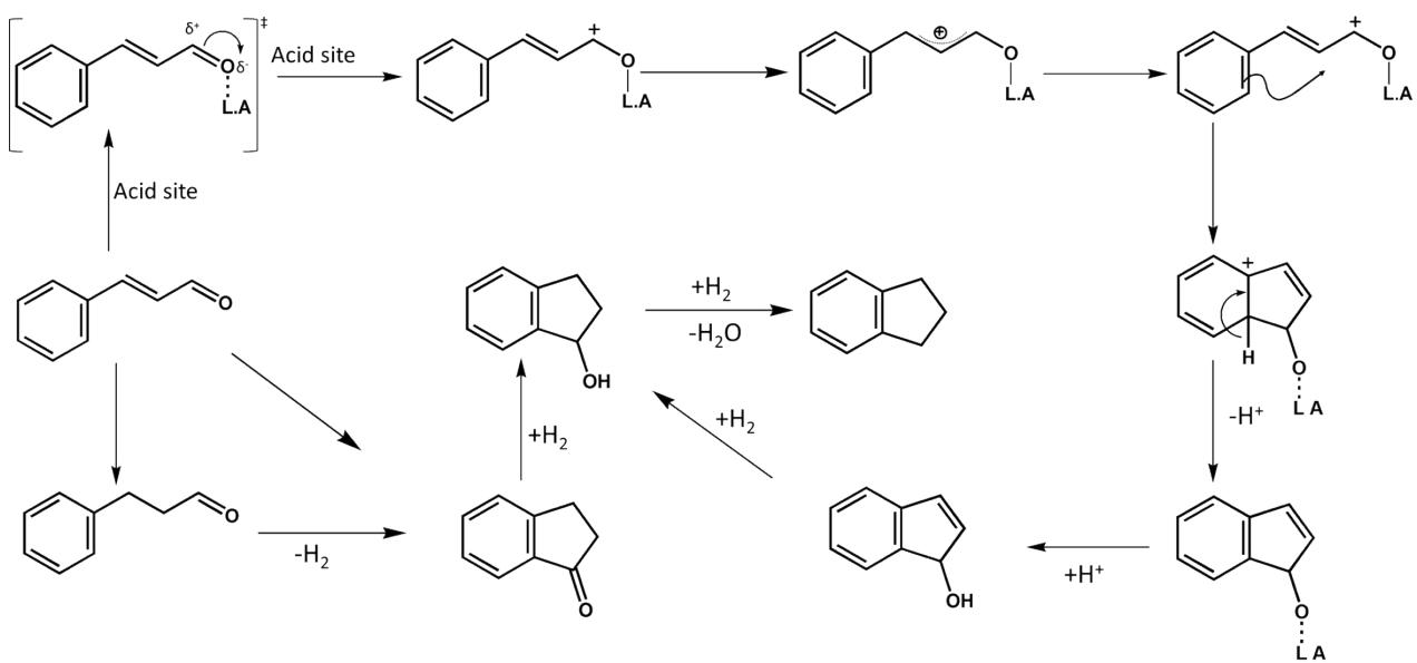
**Fig. S7** Plausible reaction mechanism of cinnamaldehyde cyclization/hydrodeoxygenation to indane derivatives.
