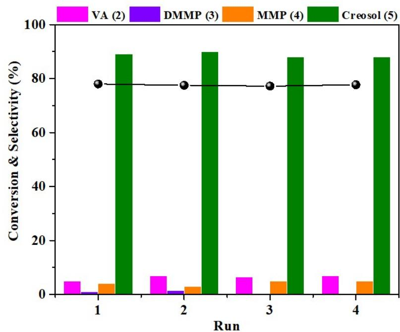
**Fig. S10** Recyclability test of the 10C-2G catalyst with high feed-to-catalyst ratio of 13.3:1 Reaction condition: 1 g vanillin, 0.075 g catalyst, 35 mL methanol, 160 °C, initial H<sub>2</sub> pressure of 1 MPa, and 2 h.
