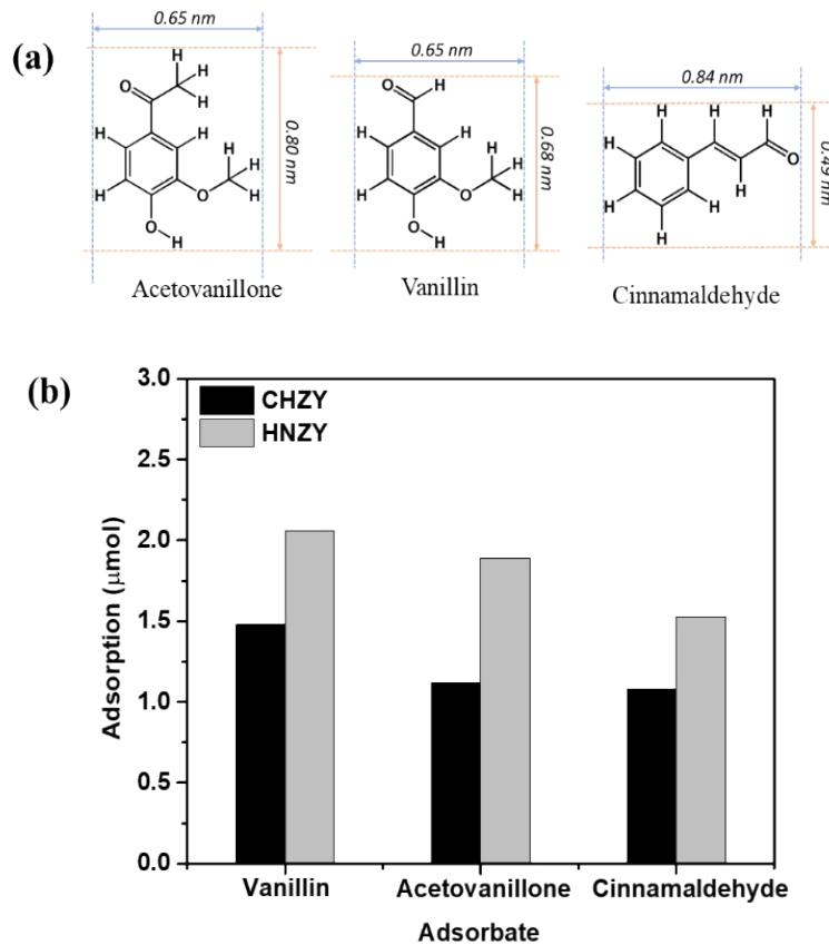
**Fig. S8** (a) Molecular size of the adsorbates calculated by the ACD/3D software and (b) adsorption study of the adsorbates with 20 mg of adsorbent (CHZY and HNZY) at room temperature. The adsorption test showed that the adsorption capacity of the adsorbates was higher in the HNZY support as compared to the C-HZY support. (Note: pore channel size of typical zeolite-Y =  $0.74 \times 0.74 \times 0.74 \text{ nm}$ )
