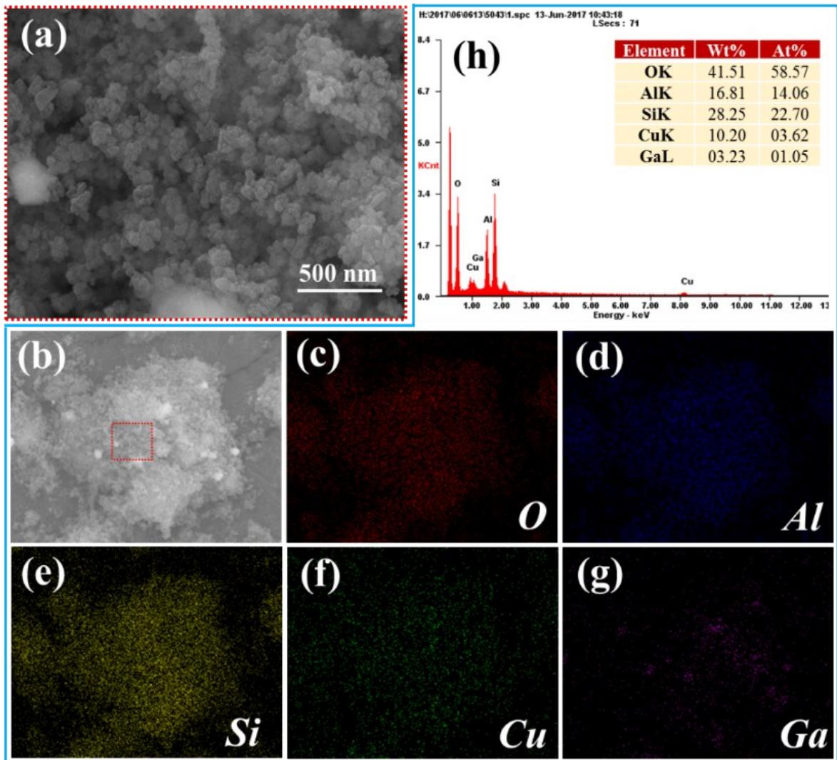
**Fig. S6** (a) FE-SEM image, (b) –(g) elemental mapping of O, Al, Si, Cu, and Ga, respectively, and (h) corresponding EDS graph of the 10C–2G catalyst.
