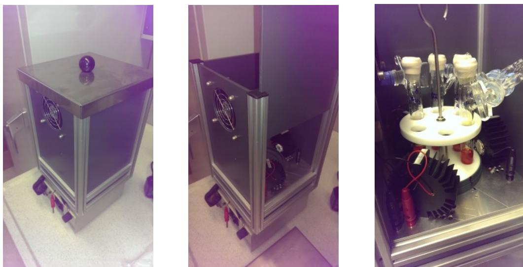
Figure S1: Pictures of the custom-made photoreactor box used for reaction performed under visible-light irradiation.
