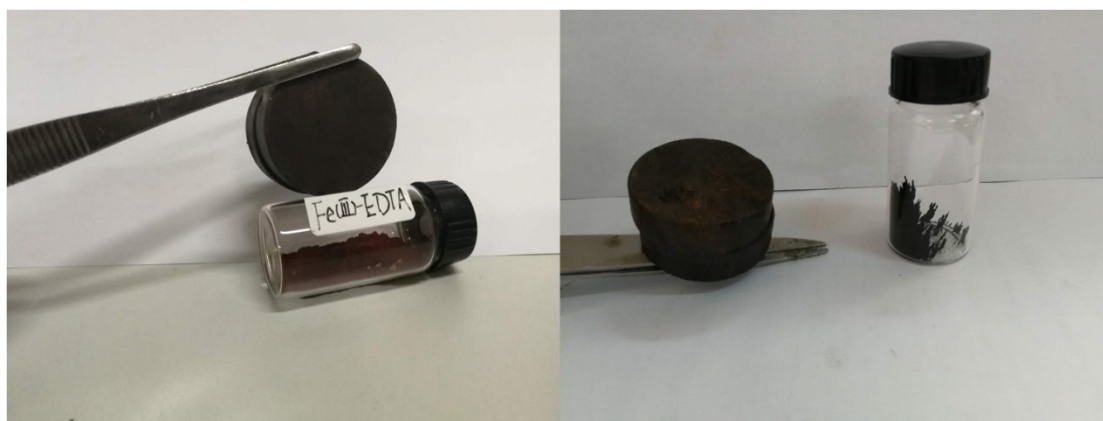
Figure S15. The magnetic properties Fe-EDTA (left) and Fe@C catalyst (right)
