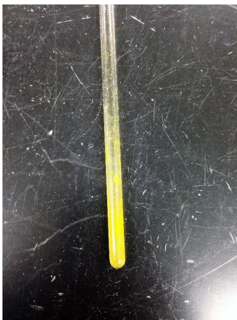
Figure S26. Image of the recovered catalyst inside the J.Young NMR tube
