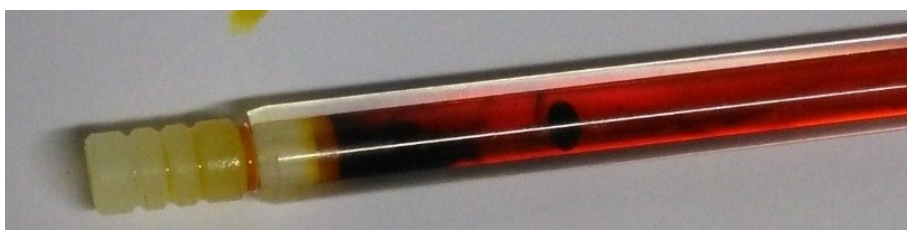
Figure S 2: Reacted viscometer sample containing [P_{44410}][Br_3] and a gold coated stainless steel ball showing signs of corrosion.
