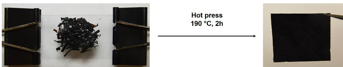
Fig. S13 Physical recycling of the cured Se-EP/Oz-Ls ( R = 1:1 ). The fragments were pressed at 190\text{ }^{\circ}\text{C} for 2 h.
