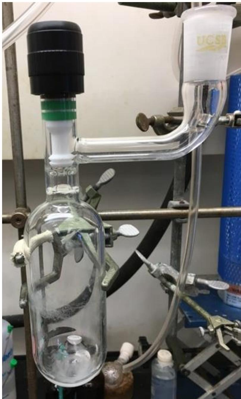
Figure S1: 400 mL threaded screwcap pressure flask.
