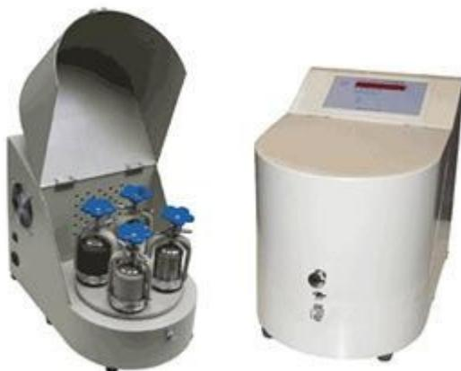
Scheme S1. The planetary ball mill used in preparation of Cu-Mn/HT.
