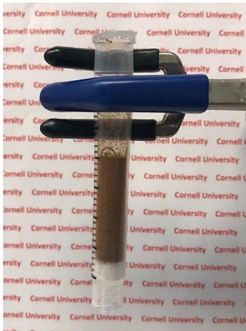
Figure S3. Breakthrough test set-up using a 3 mL syringe filled with 100 mg of HNTs@Fe-PAPTMAC.
