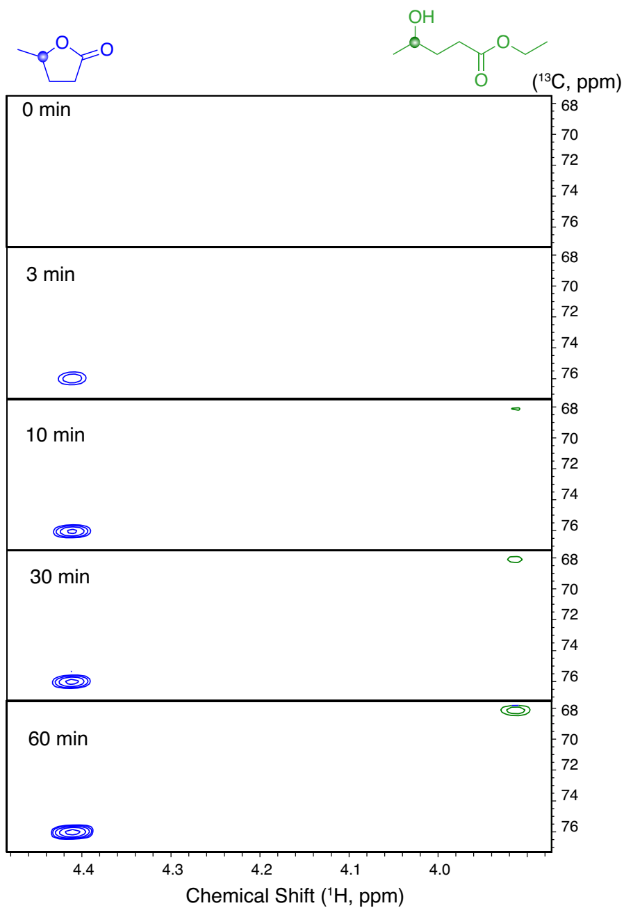
Fig. S12. Ex situ NMR spectra of the reaction mixture in the region for the intermediate (ethyl 4-hydroxypentanoate, EHP) and product ( \gamma -valerolactone, GVL). After the indicated reaction times, the reaction mixture was quenched by methanol at room temperature and then sent for NMR analysis. Clearly, better selectivity was observed for the product here than in the NMR tube (Fig. S11).
