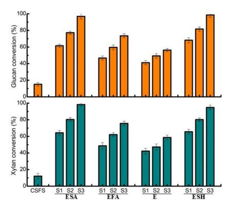
Electronic supplemental information C Correlations between the glucan/xylan conversion and removal rates of xylan and lignin. ESA represents ethanol plus sulfuric acid; EFA represents ethanol plus formic acid; ESH represents ethanol plus sodium hydroxide. S1, S2 and S3 represent stage 1, stage 2 and stage 3, respectively
