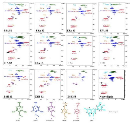
Electronic supplemental information H <sup>31</sup>P-NMR spectra of the fractionated lignin produced from each sequential organosolv fragmentation approach (SOFA). ESA represents ethanol plus sulfuric acid; EFA represents ethanol plus formic acid; ESH represents ethanol plus sodium hydroxide. S1, S2 and S3 represent stage 1, stage 2 and stage 3, respectively
