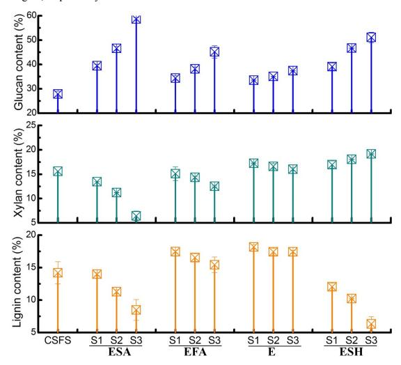
Electronic supplemental information B Enzymatic hydrolysis of pretreated solids by sequential organosolv fragmentation approach (SOFA). Fragmentation approaches are described in Table 1. CSFS stands for corn stover feedstock. ESA represents ethanol plus sulfuric acid; EFA represents ethanol plus formic acid; ESH represents ethanol plus sodium hydroxide. S1, S2 and S3 represent stage 1, stage 2 and stage 3, respectively
