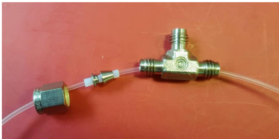
Figure S8: Tee piece used in the continuous downstream.
