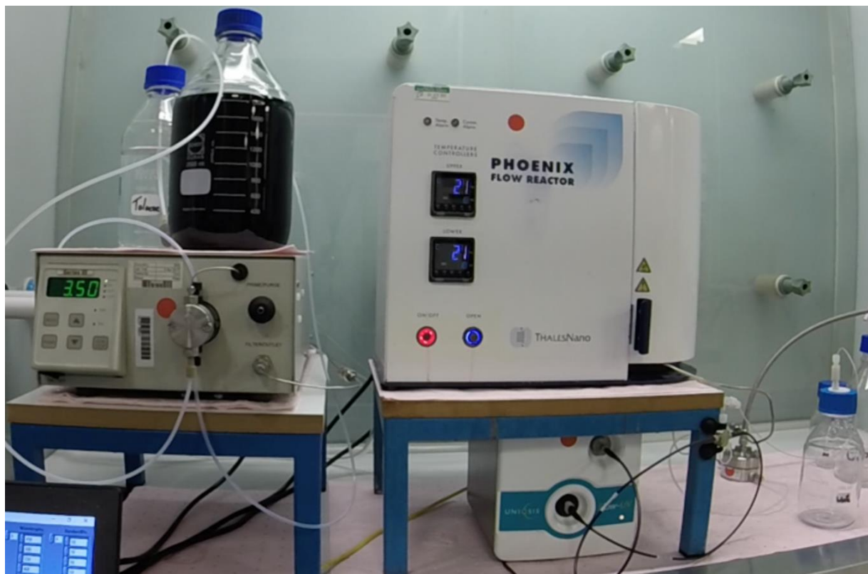
Figure S1: System composed by Series III HPLC pump, Phoenix reaction, Equilibar back pressure regulator and FlowUV.
