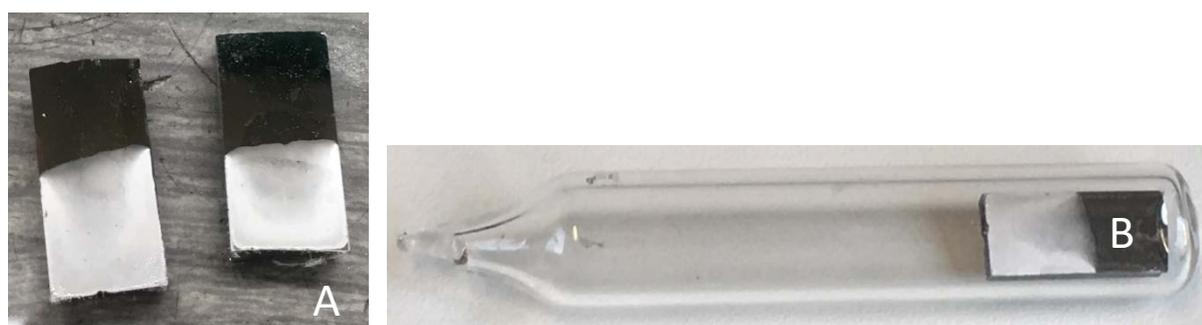
**Fig. S15** Indium deposits on a molybdenum working electrode from an  $\text{InCl}_3$  aqueous bath by using a high current density of  $250\text{ mA cm}^{-2}$  and a low deposition-bath temperature of  $-5^\circ\text{C}$  unfused (A) and fused in glass under vacuum (B).
