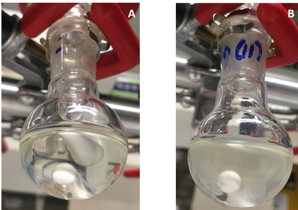
**Fig. S7** Purified Cyphos IL 101 containing 30 mM of indium(I) (A) and 30 mM of indium(II) (B). A small piece of solid grey material can be observed on the bottom of the flask.
