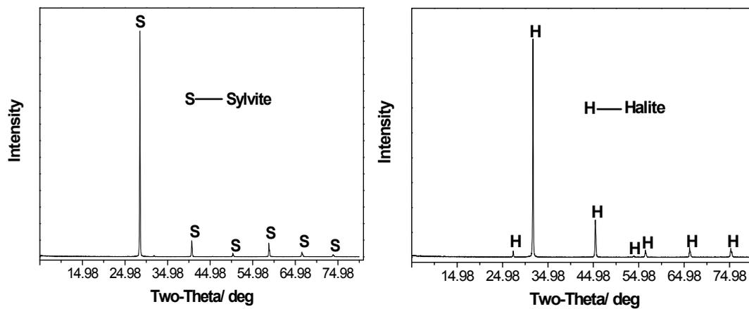
**Figure S1.** XRD of KCl (sylvite) and NaCl (halite)
