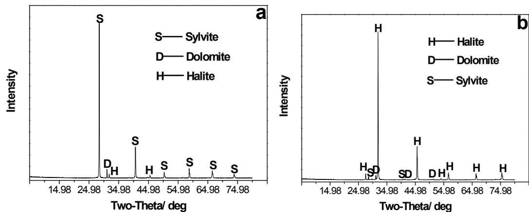
**Figure S3.** XRD of the recovered KCl concentrate (a) and NaCl tailing (b) using Gemini surfactant BOBD
