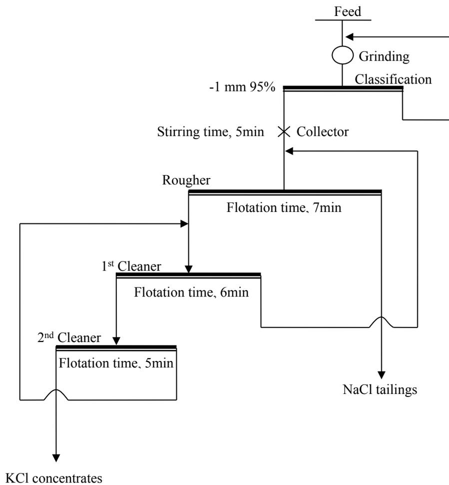
**Figure S2.** The flowsheet of froth flotation experiments
