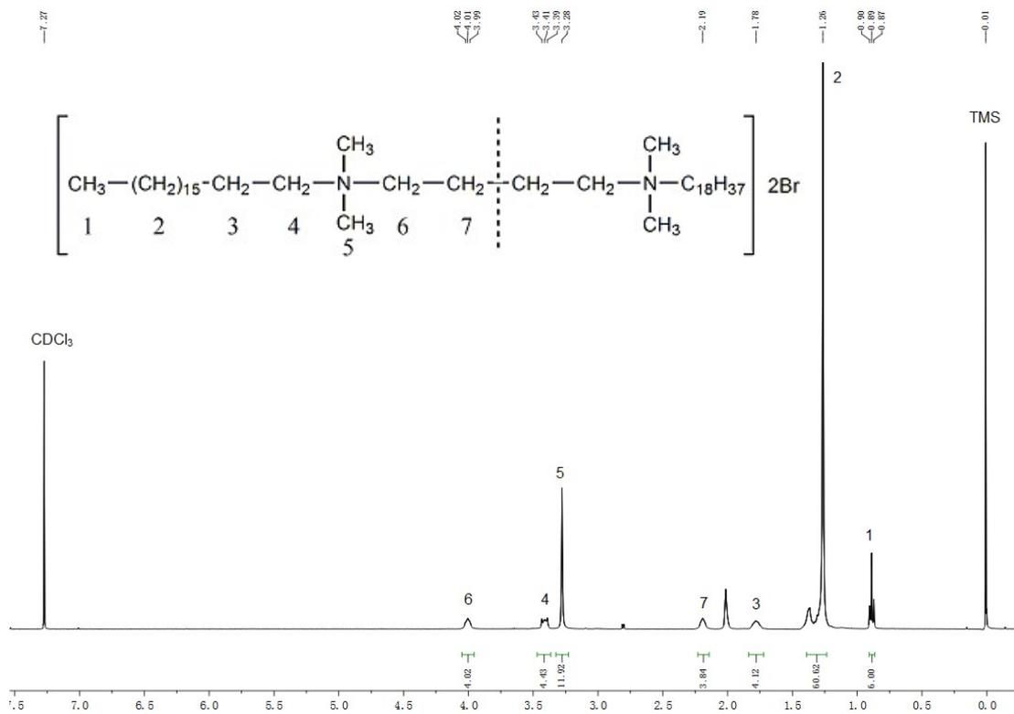
**Figure S7.** <sup>1</sup>H NMR spectra of Gemini surfactant BOBD in CDCl<sub>3</sub>
