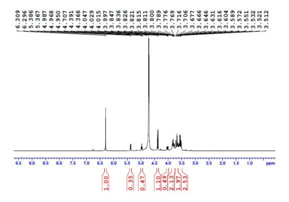
$^1\text{H}$  NMR of the recation between D-(+)- ribose and malononitrile in presence of 15 mol%  $K_3PO_4$  after 4 h in  $D_2O$
