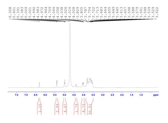
$^1\text{H}$  NMR of the recation between D-(+)- ribose, malononitrile with  $K_2CO_3$  (15 mol%) in D\_2O after180 minutes
