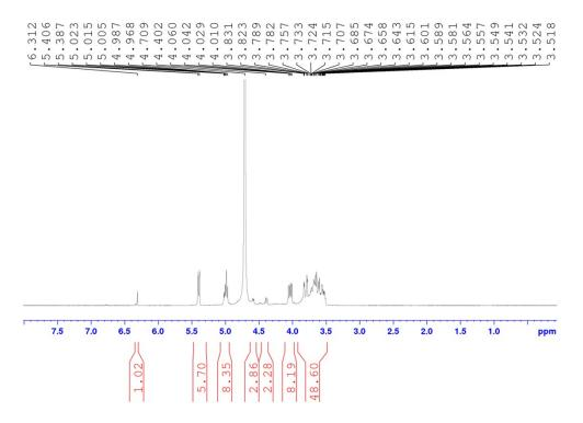
$^{1}$ H NMR of the recation between D-(+)- ribose, malononitrile with K<sub>2</sub>CO<sub>3</sub> (15 mol%) in D<sub>2</sub>O after100 minutus
