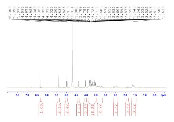
$^1\text{H}$  NMR of the recation between D-(+)- ribose, malononitrile with DBU (15 mol% ) in D\_2O after 140 minutes
