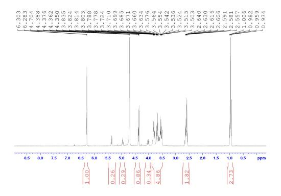
$^{1}$ H NMR of the recation between D-(+)- ribose and malononitrile in presence of 5 mol% Et<sub>3</sub>N after 4 h in D<sub>2</sub>O
