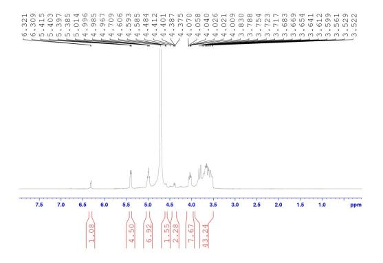
$^1\text{H}$  NMR of the recation between D-(+)- ribose, malononitrile with  $K_2CO_3$  (15 mol%) in D\_2O after140 minutes
