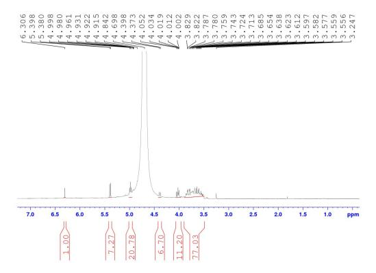
$^1\text{H}$  NMR of the recation between D-(+)- ribose and malononitrile in presence of 10 mol% Et\_3N after 4 h in D\_2O
