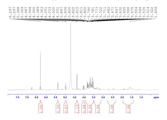
$^{1}$ H NMR of the recation between D-(+)- ribose, malononitrile with K<sub>2</sub>CO<sub>3</sub> (15 mol%) in D<sub>2</sub>O after 20 minutus
