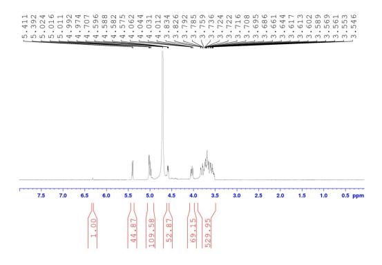
$^{1}$ H NMR of the recation between D-(+)- ribose, malononitrile with K<sub>2</sub>CO<sub>3</sub> (15 mol%) in D<sub>2</sub>O after 60 minutus
