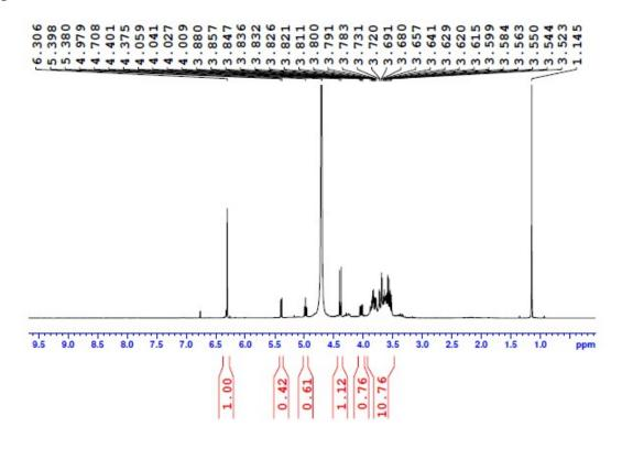
$^{1}$ H NMR of the recation between D-(+)- ribose and malononitrile in presence of 15 mol% Me<sub>3</sub>N after 4 h in D<sub>2</sub>O
