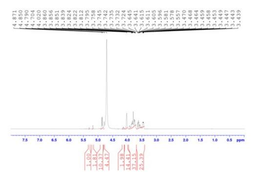
$^{1}H$  NMR of the recation between D-(+)- ribose and malononitrile in presence of Yb(OTf)<sub>3</sub> in D<sub>2</sub>O
