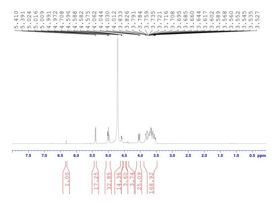
$^1\text{H}$  NMR of the recation between D-(+)- ribose, malononitrile with  $K_2\text{CO}_3$  (15 mol% ) in D\_2O after 80 minutus
