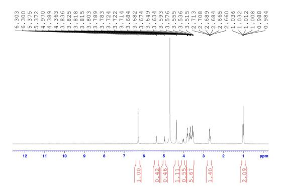
$^{1}$ H NMR of the recation between D-(+)- ribose and malononitrile in presence of 15 mol% CsCO<sub>3</sub> after 4 h in D<sub>2</sub>O
