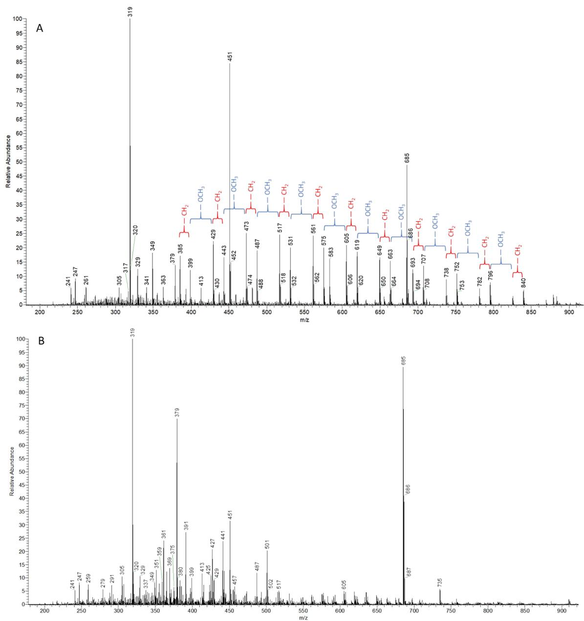
**Fig S4** SEC-ESI spectra of oil from bagasse liquefaction without catalyst (A) and with Pd/C catalyst (B) in methanol for 8 h. The peak at 685.43 associated with the solvent THF used for ESI analysis.
