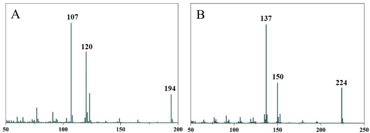
**Fig. S3** Mass spectrum of A) ethyl 3-(4-hydroxyphenyl) propanoate and B) ethyl 3-(3-hydroxy-4-methoxyphenyl) propanoate from direct depolymerisation of sugarcane bagasse in ethanol.
