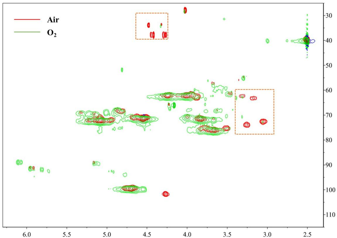
**Fig S13** Comparison of 2D HSQC NMR spectra of solid residue obtained from direct conversion of bagasse under O<sub>2</sub> (green line) and air (red line) atmosphere.
