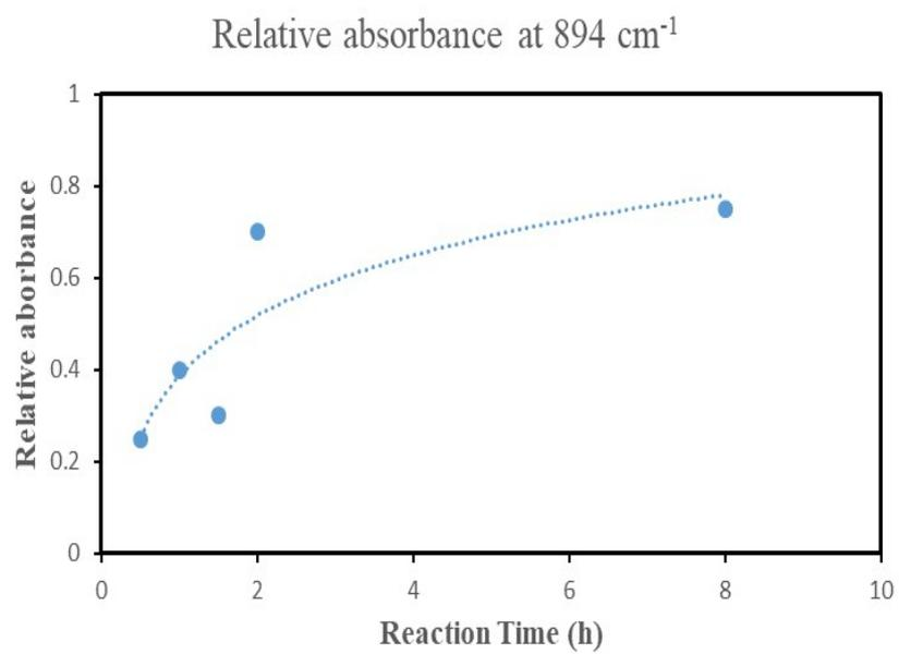
**Fig S10** Relative absorbance at 894  $\text{cm}^{-1}$  for oil fractions obtained with different reaction time.
