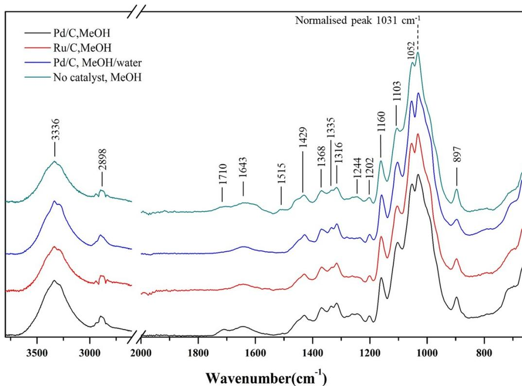
**Fig. S11** FTIR spectra of solid residue from bagasse liquefaction under different reaction conditions.
