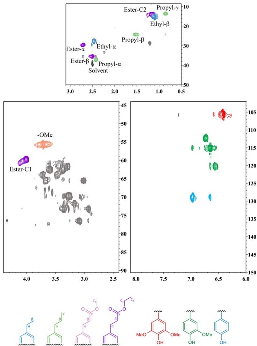
**Figure S8** 2D NMR spectrum of oil obtained from delignification of sugarcane bagasse with Pd/C and ethanol used as solvent.
