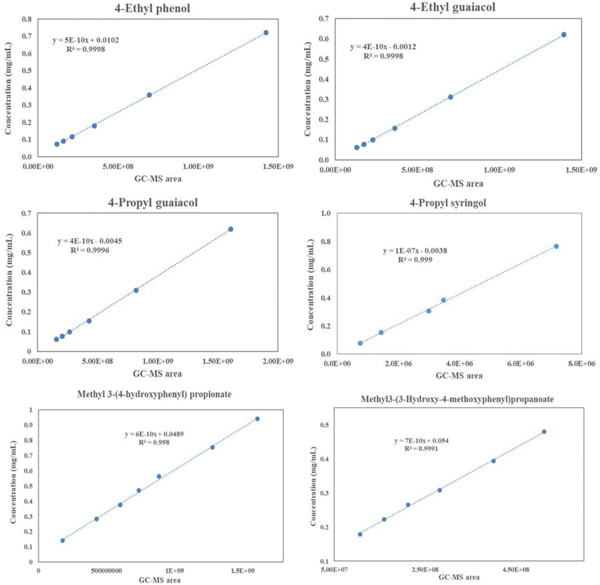
**Fig. S2** GC-MS calibration curve of main aromatic components from direct depolymerisation of sugarcane bagasse based on commercial standards.
