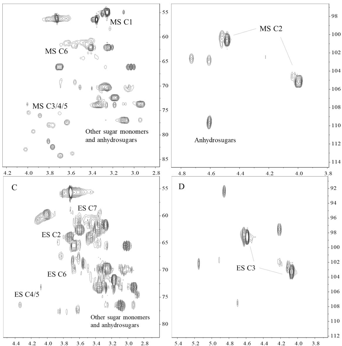
**Fig S12** 2D HSQC NMR spectra of the chemical correlation in the structure of mono-sugars alcohol derivatives from hemicellulose. A and B present for methylated mono-sugars, C and D present for the ethylated mono-sugars, C1-7 refer to the carbon position in the sugar derivatives structure.
