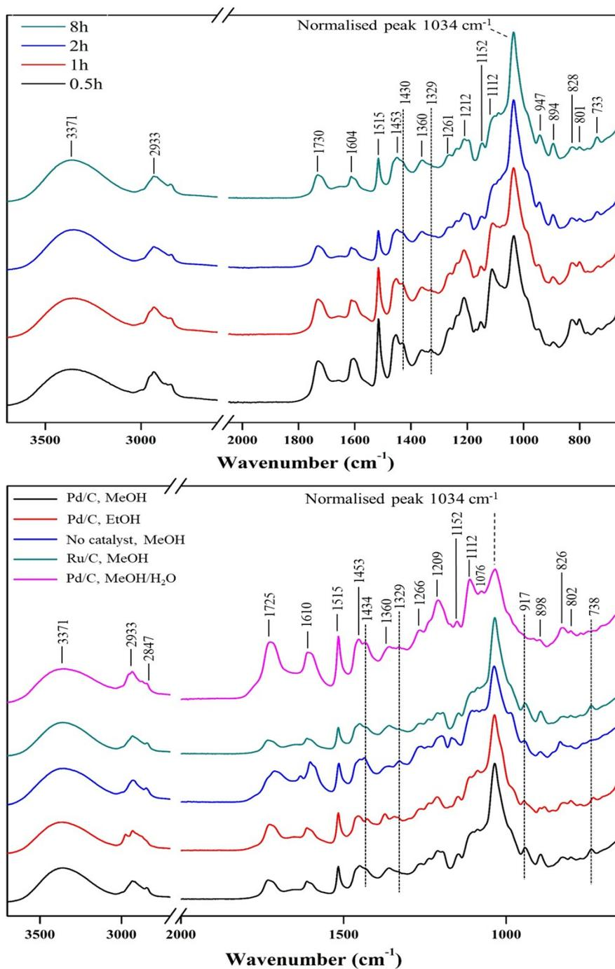
**Fig S9** FTIR spectra of oil products obtained under different reaction time (0.5 h -8 h) and different reaction conditions.
