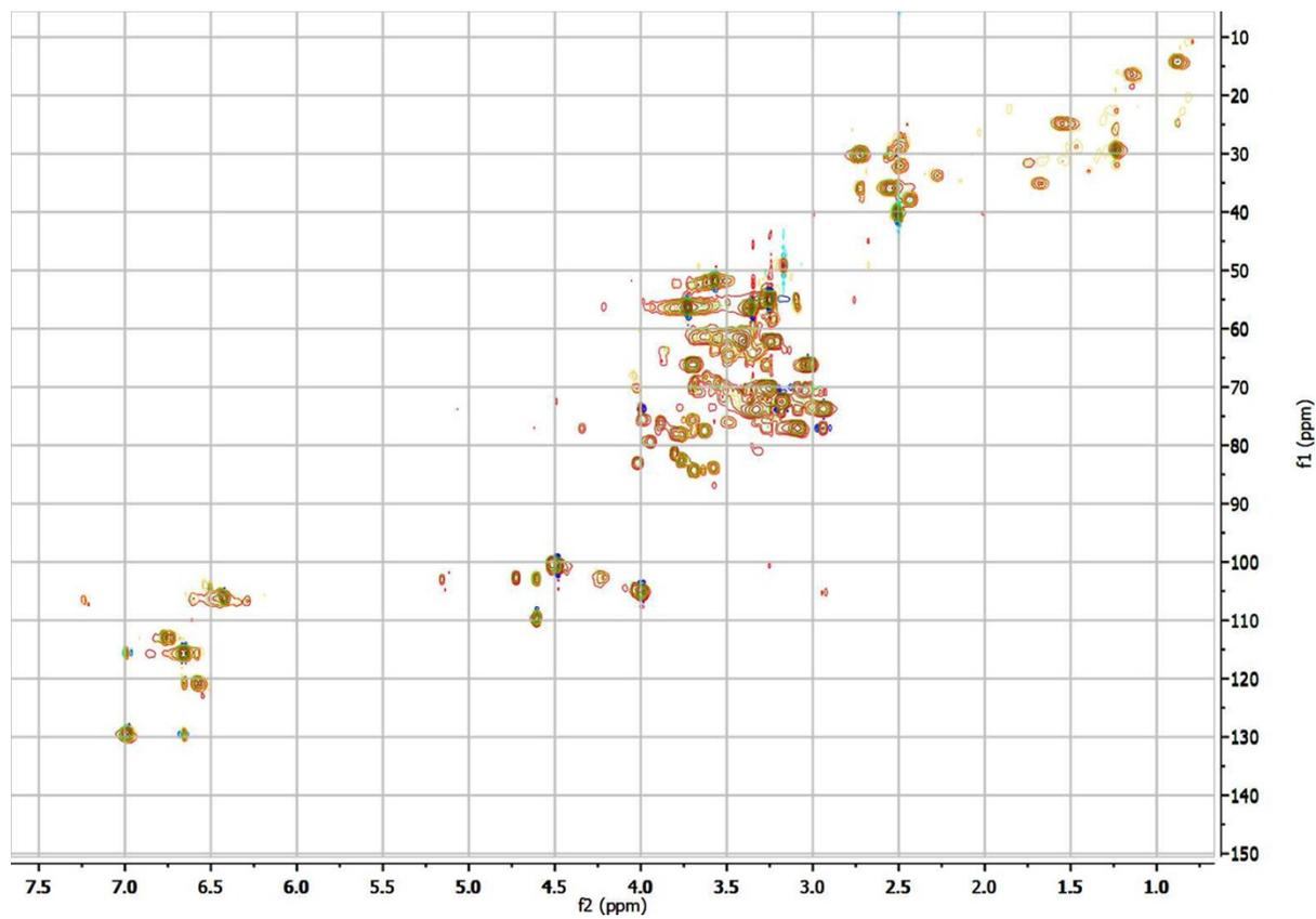
**Fig S14** Comparison of 2D HSQC NMR spectra of oil fraction obtained from direct conversion of bagasse under O<sub>2</sub> (green line), Ar (yellow line) and air (red line).
