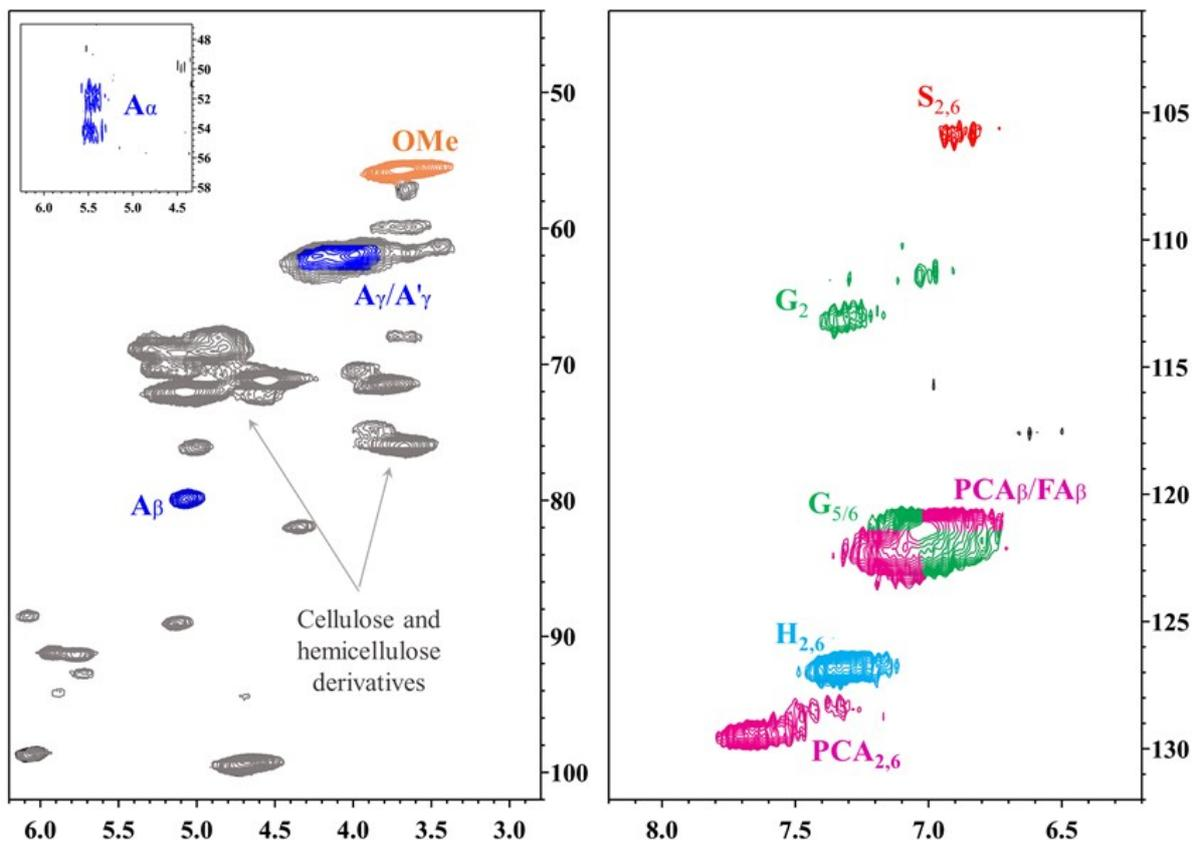
**Figure S6** 2D NMR spectra of sugarcane trash.
