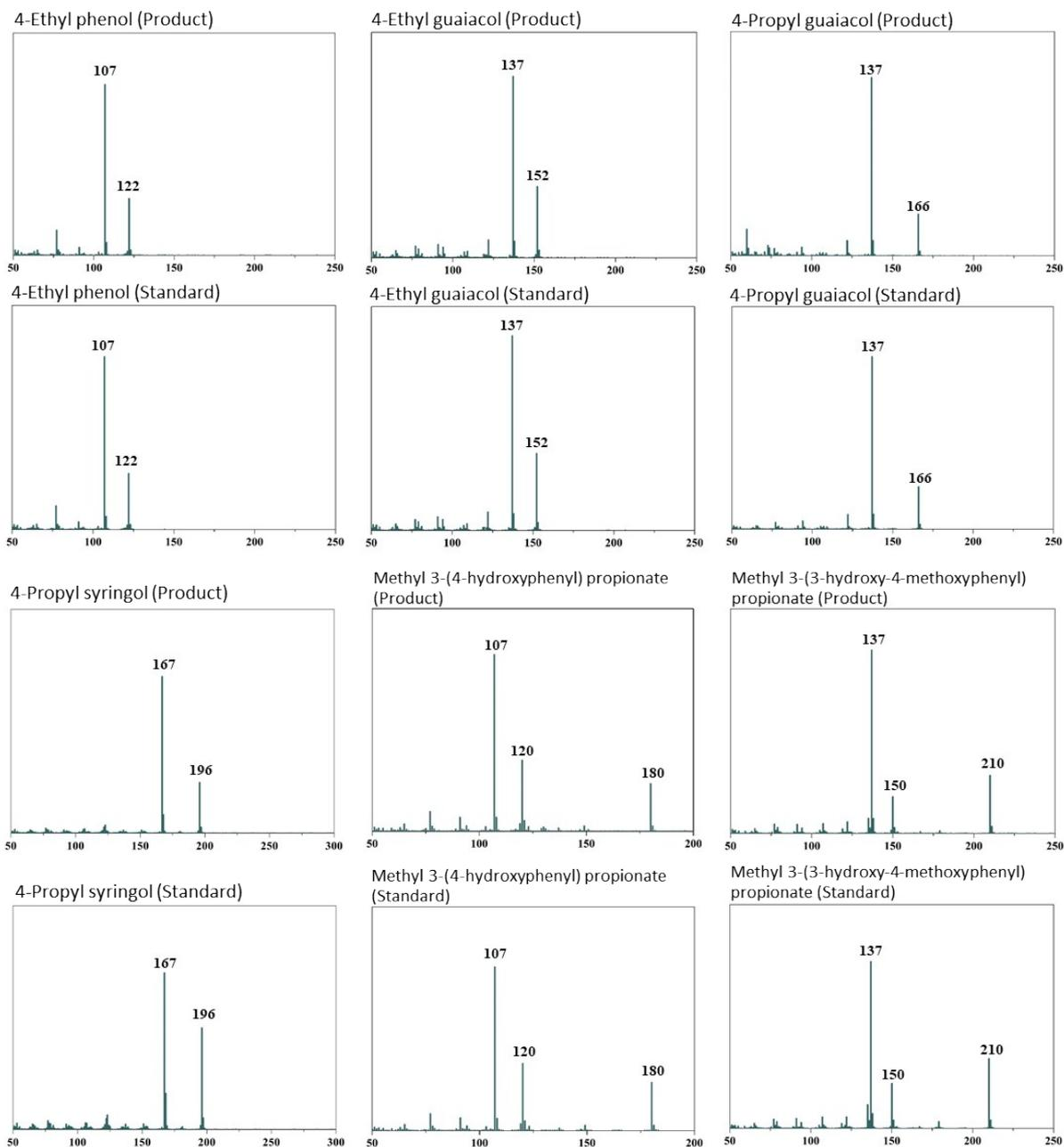
**Fig. S1** Mass spectrum of the main aromatic components from direct depolymerisation of sugarcane bagasse in methanol and their commercial standards.
