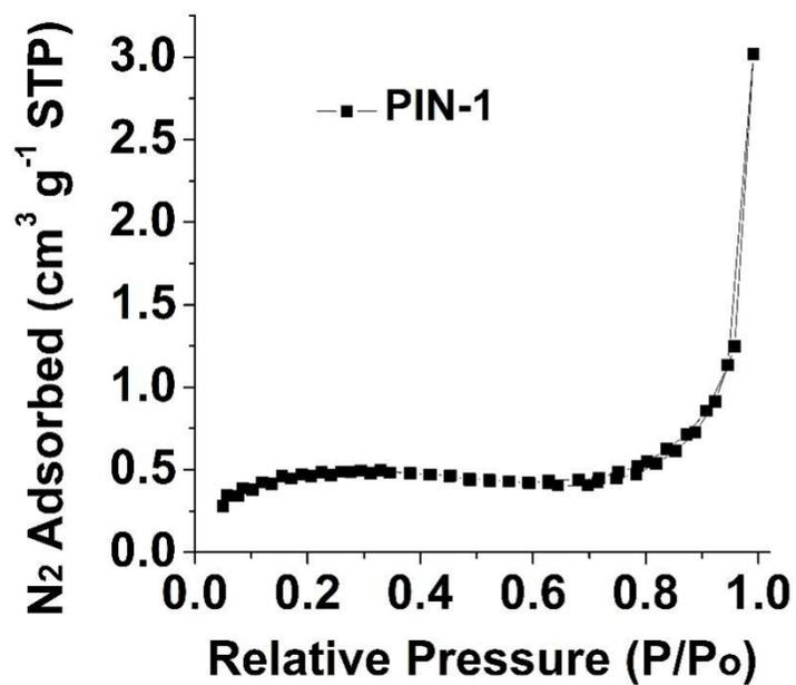
Figure S2. The N<sub>2</sub> sorption isotherm (77K) of PIN-1 material.
