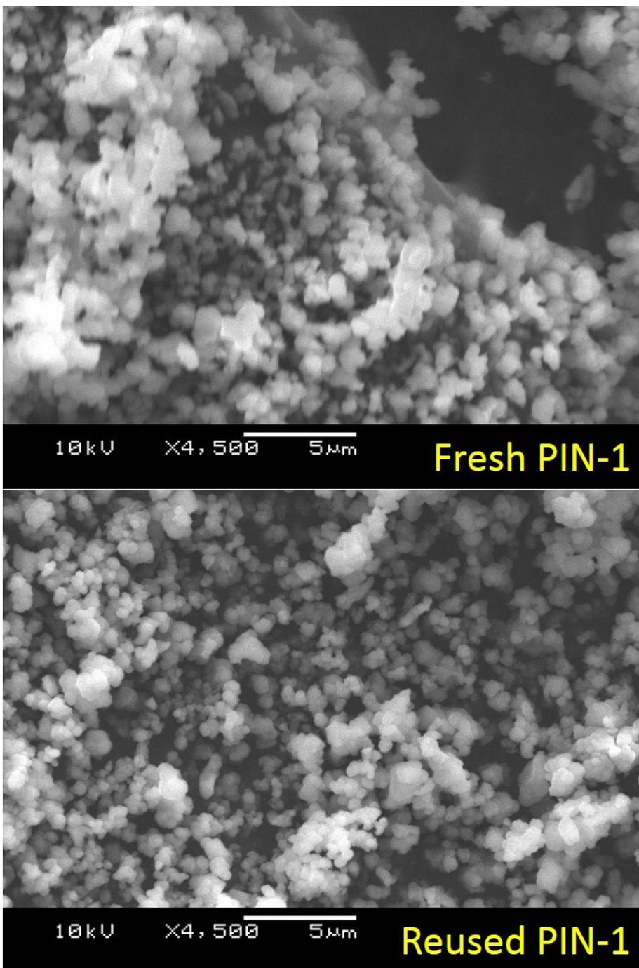
**Figure S3.** SEM images of Fresh and Recycled PIN-1 catalyst.
