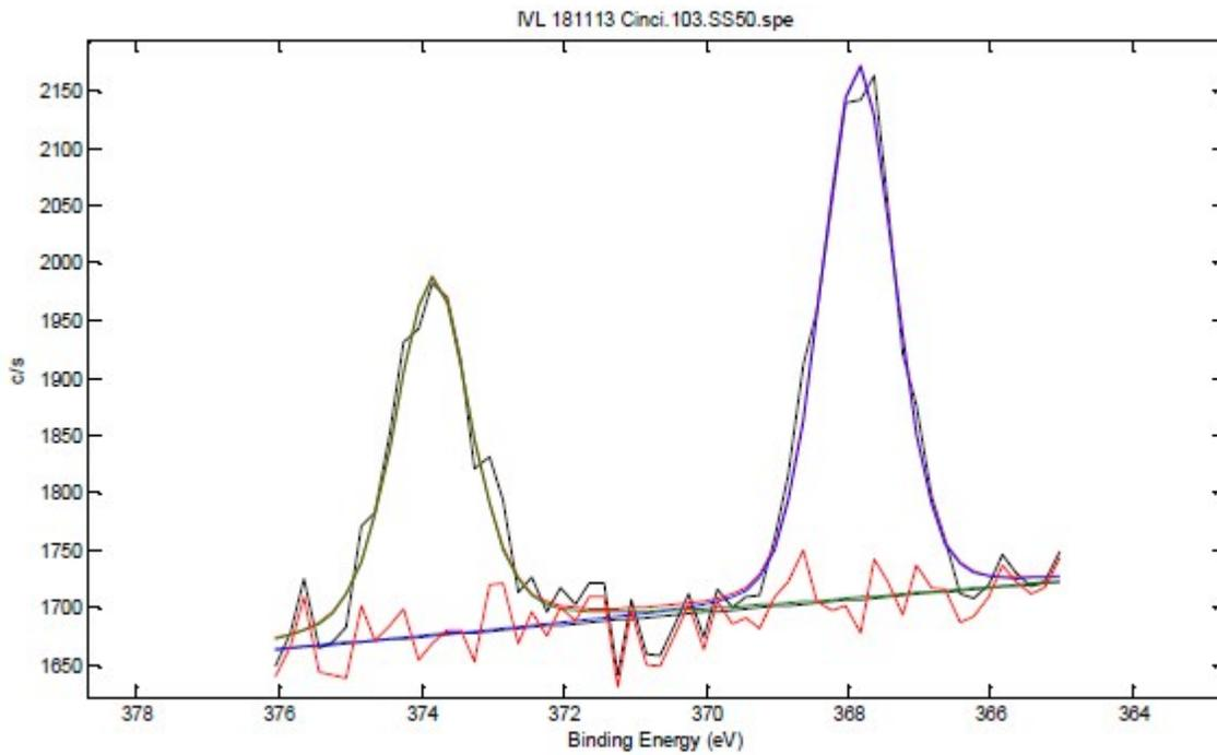
**Figure S8.** Detailed XPS analysis for AgPd/Fe@CN<sub>x</sub> catalyst. c) O1s spectra. d) Ag3d spectra
