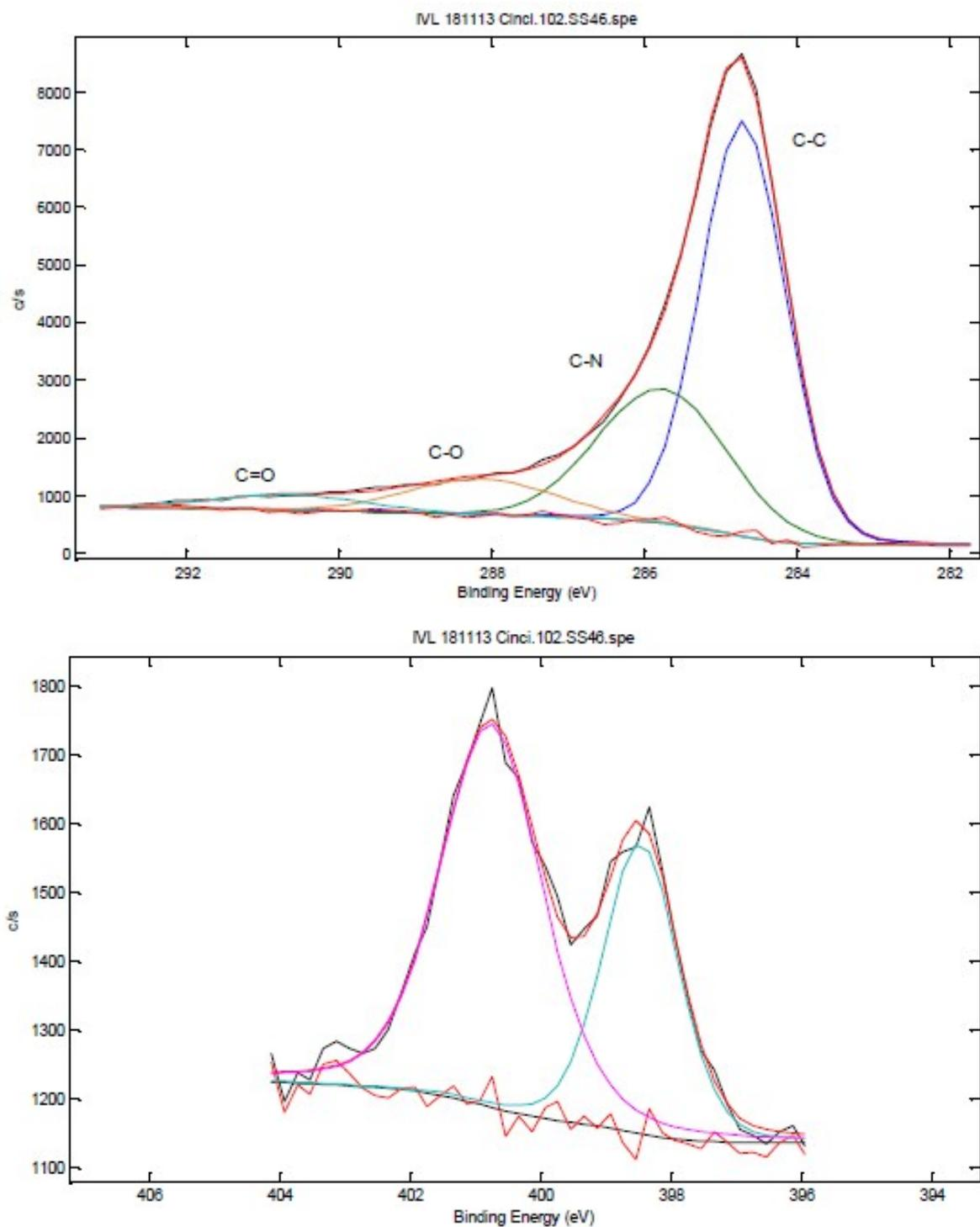
**Figure S6.** Detailed XPS analysis for carbon nitride (CN<sub>x</sub>) catalyst. a) C1s spectra. b) N1s spectra.
