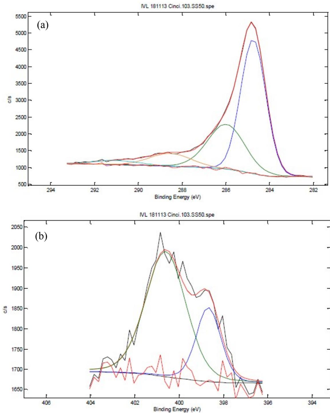
**Figure S7.** Detailed XPS analysis for AgPd/Fe@CN<sub>x</sub> catalyst. a) C1s spectra. b) N1s spectra.
