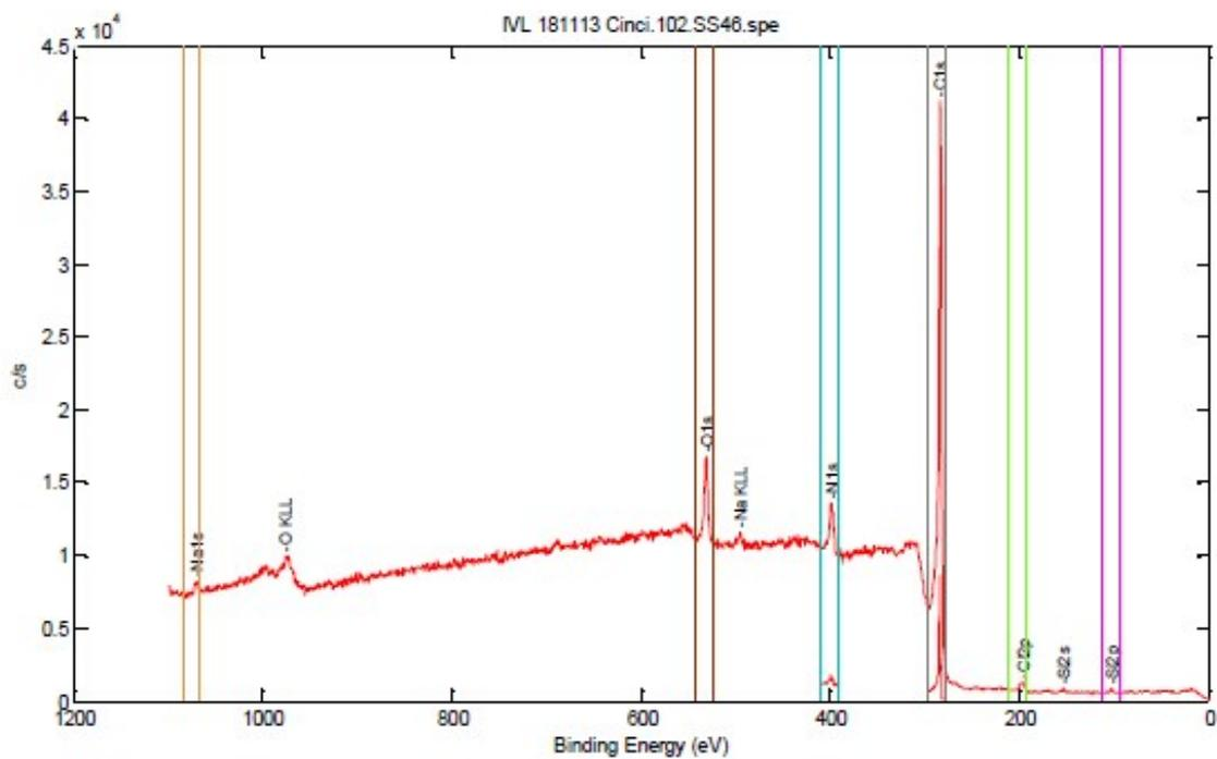
**Figure S4.** XPS full spectrum of carbon nitride (CN<sub>x</sub>)
