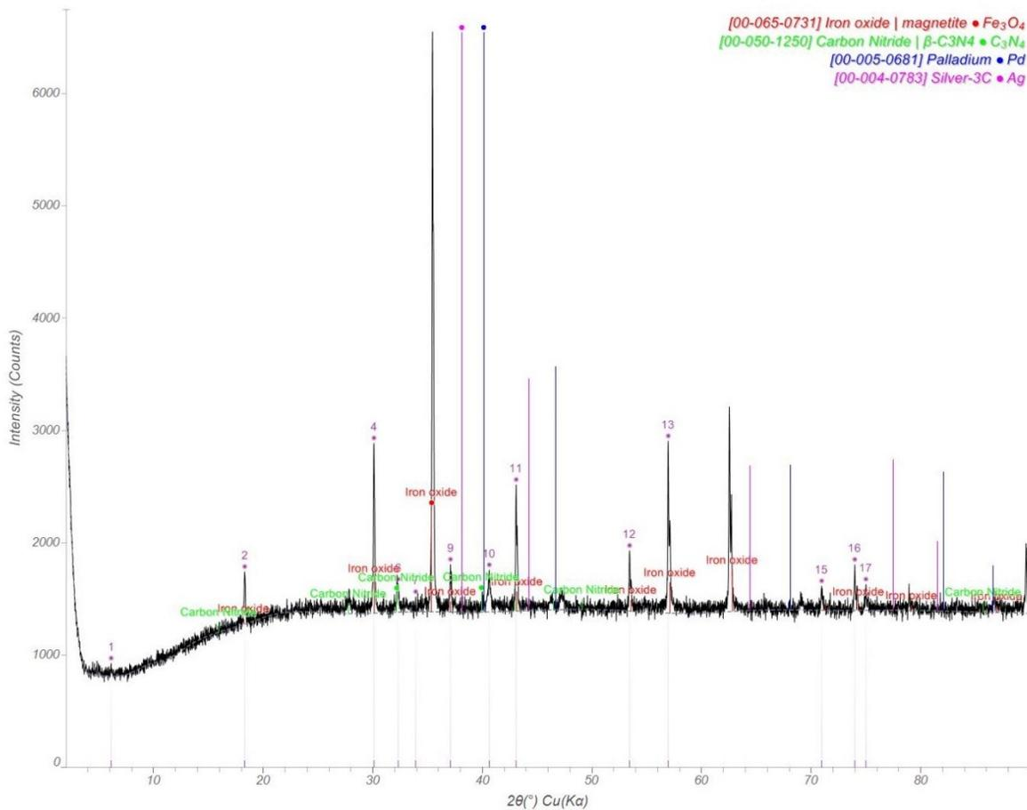
**Figure S3.** XRD analysis of AgPd/Fe@CN<sub>x</sub> as compared with JCPDS standards
