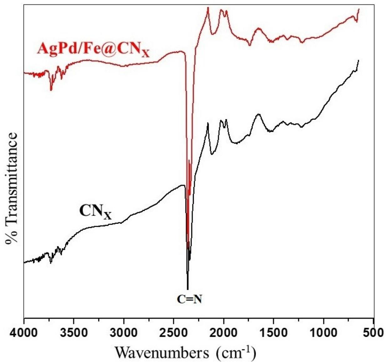
Figure S10. FT-IR of CN<sub>x</sub> and AgPd/Fe@CN<sub>x</sub> catalyst
