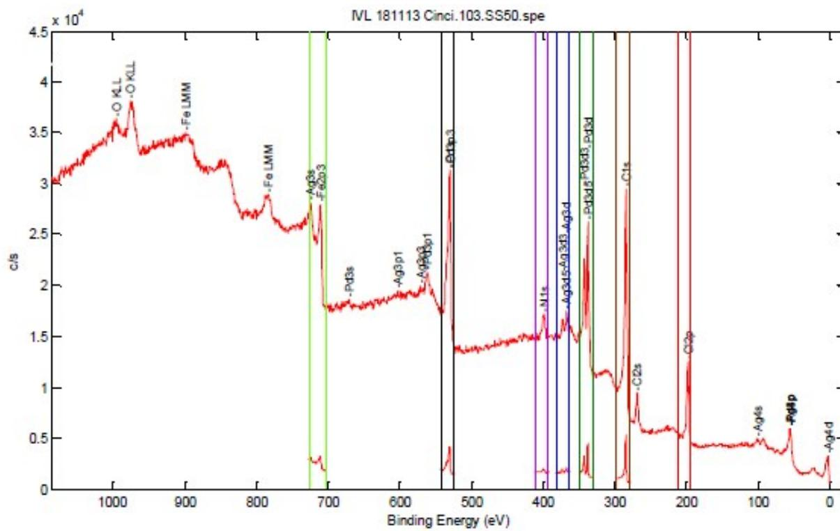
**Figure S5.** XPS full spectrum of AgPd/Fe@CN<sub>x</sub>
