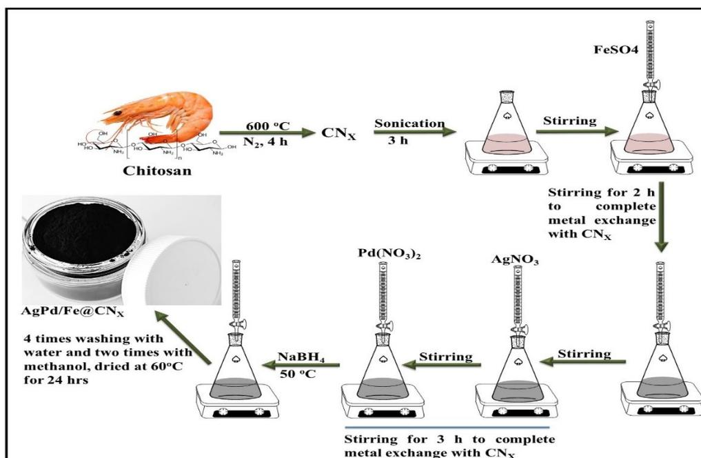
Figure S1: Pictorial representation of the synthesis of  $AgPd/Fe@CN_x$
