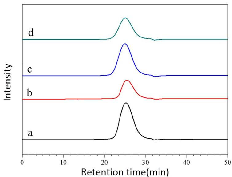
**Figure S2** GPC chart of SMA obtained after 3 h (a), 5 h (b), 7 h (c) and 9 h (d) of reaction respectively (reaction condition: catalyst (n (DETA & NaOH), 0.2 mol; n (DETA/NaOH), 6/1), atmospheric pressure, 100°C).
