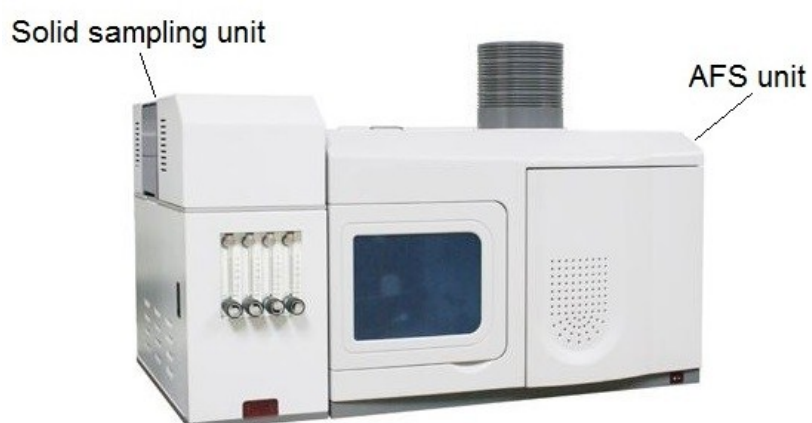
32 Figure S1 The full picture of the solid sampling Hg-Cd analyzer.
