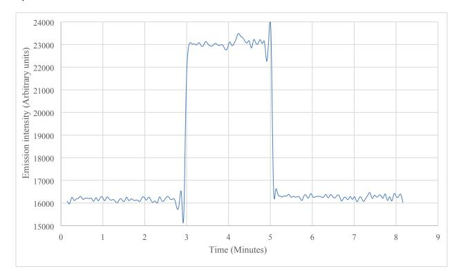
SF 2: Au (I) 267.595 spectra of 2-ethylhexanol gold solution being aspirated in and washed out of the MP-4100 by 3 M HCl extract
