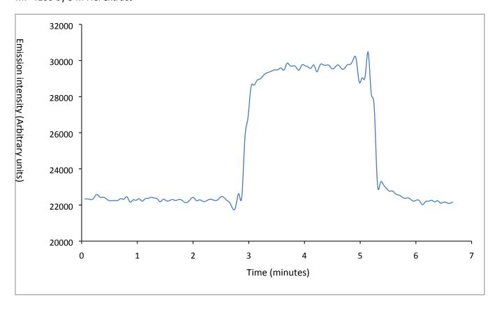
SF 3: Au (I) 267.595 spectra of MIBK gold solution being aspirated in and washed out of the MP-4100 from a 1 M HCl extract
