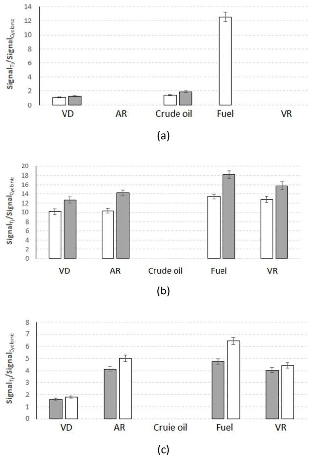
**Figure S1.** Peak height found with the hTISIS normalized with respect to that measured for the Cyclonic reference spray chamber. (a) Vanadium; (b) iron; (c) aluminum. White bars: hTISIS temperature: 200 °C; grey bars: hTISIS temperature: 400 °C. Samples dilution factor: 1:10
