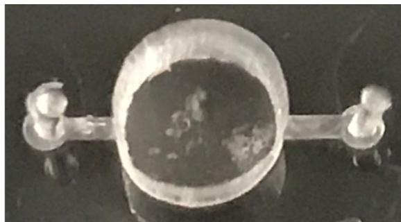
**Fig. S1** Photograph of on-chip reaction cavity with no reagent inside (a) and after water evaporation (b).
