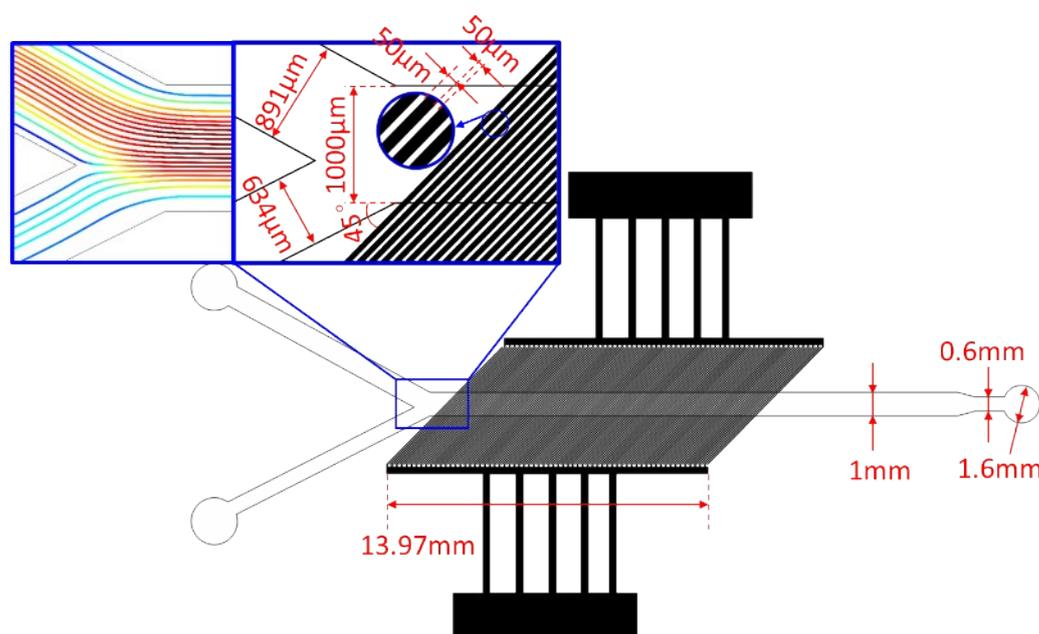
Fig. S1 Layout of the chip and simulated streamlines of the laminar flow in the down-stream of the chip.
