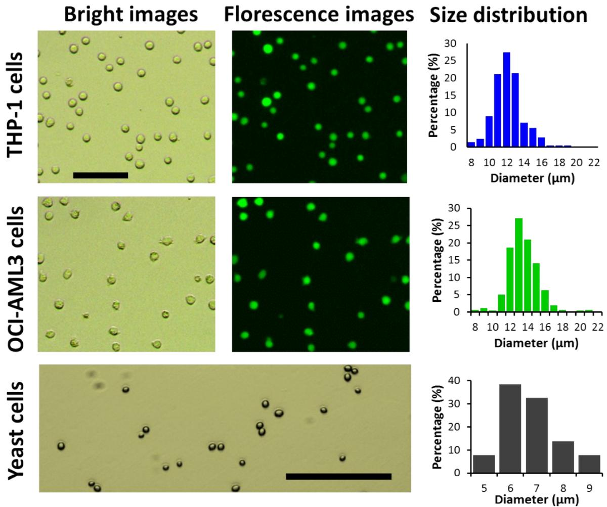
Fig. S4 Measured size distribution of the cells used in this paper. Scale bar=100  $\mu\text{m}$ .
