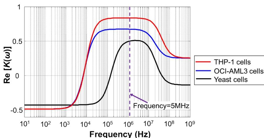
**Fig. S6** Real part of the CM factor of THP-1, OCI-AML3 and yeast cells. For those three types of cells,  $\text{Re}[K(\omega)] > 0$  at the working frequency of 5MHz, which means that all those cells experienced positive DEP force.
