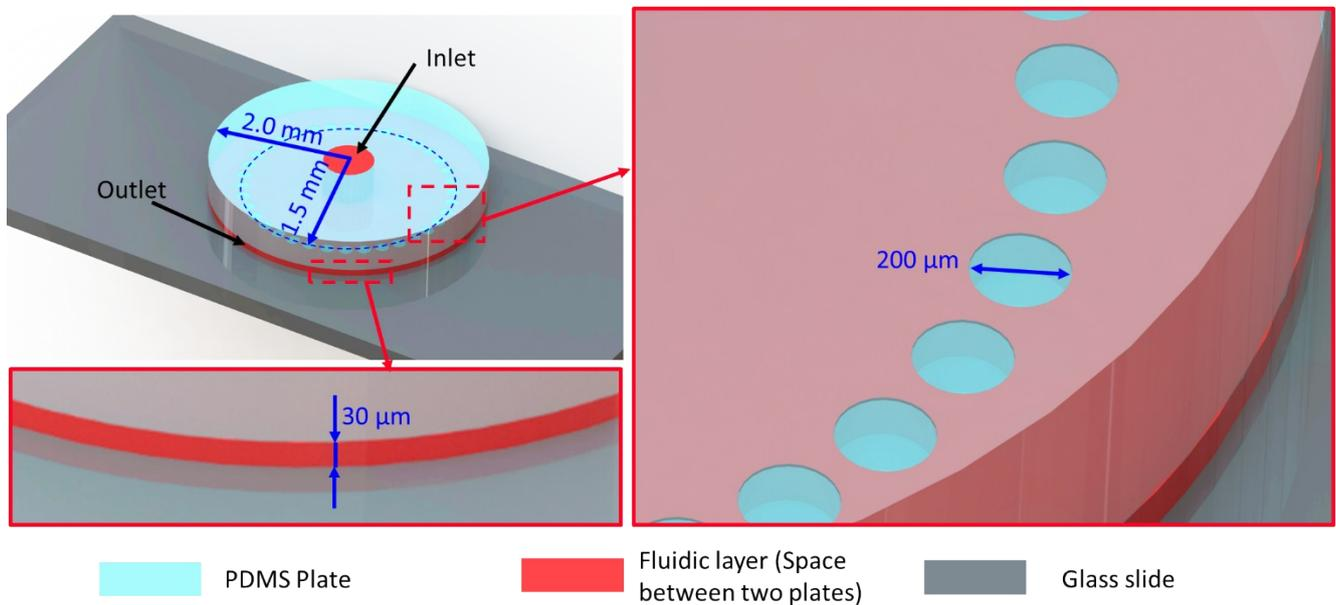
Fig. S5 Schematics of the designed microfluidic chip with an inlet and a 360°-opened outlet for study gravitational sedimentation of cells in the tubing (Fig. 3). The outlet is a circular space sandwiched by two plates. The upper plate is a PDMS plate with pillars which have the diameter of 200- $\mu\text{m}$  and the bottom plate is a glass slide. They are bonded together by the treatment of oxygen plasma. The pillars of the upper PDMS plate are the supports between two plates.
