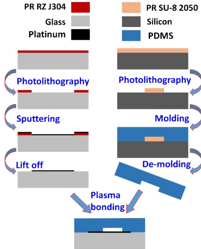
Fig. S2 Schematic of the chip fabrication process.
