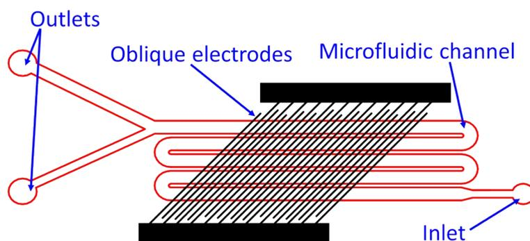
**Fig. S7 Schematic of the chip design for increasing the throughput of DEP separation through extending the flow path in the DEP region.**
