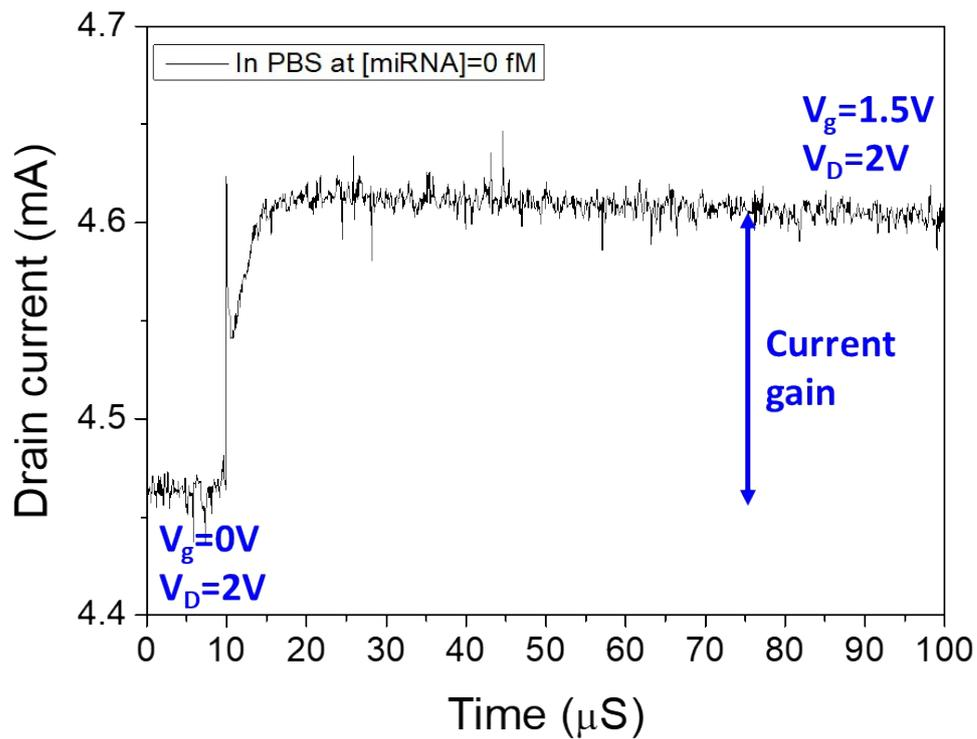
Supplementary figure S4. Typical drain current response of AlGaN/GaN HEMT sensor.
