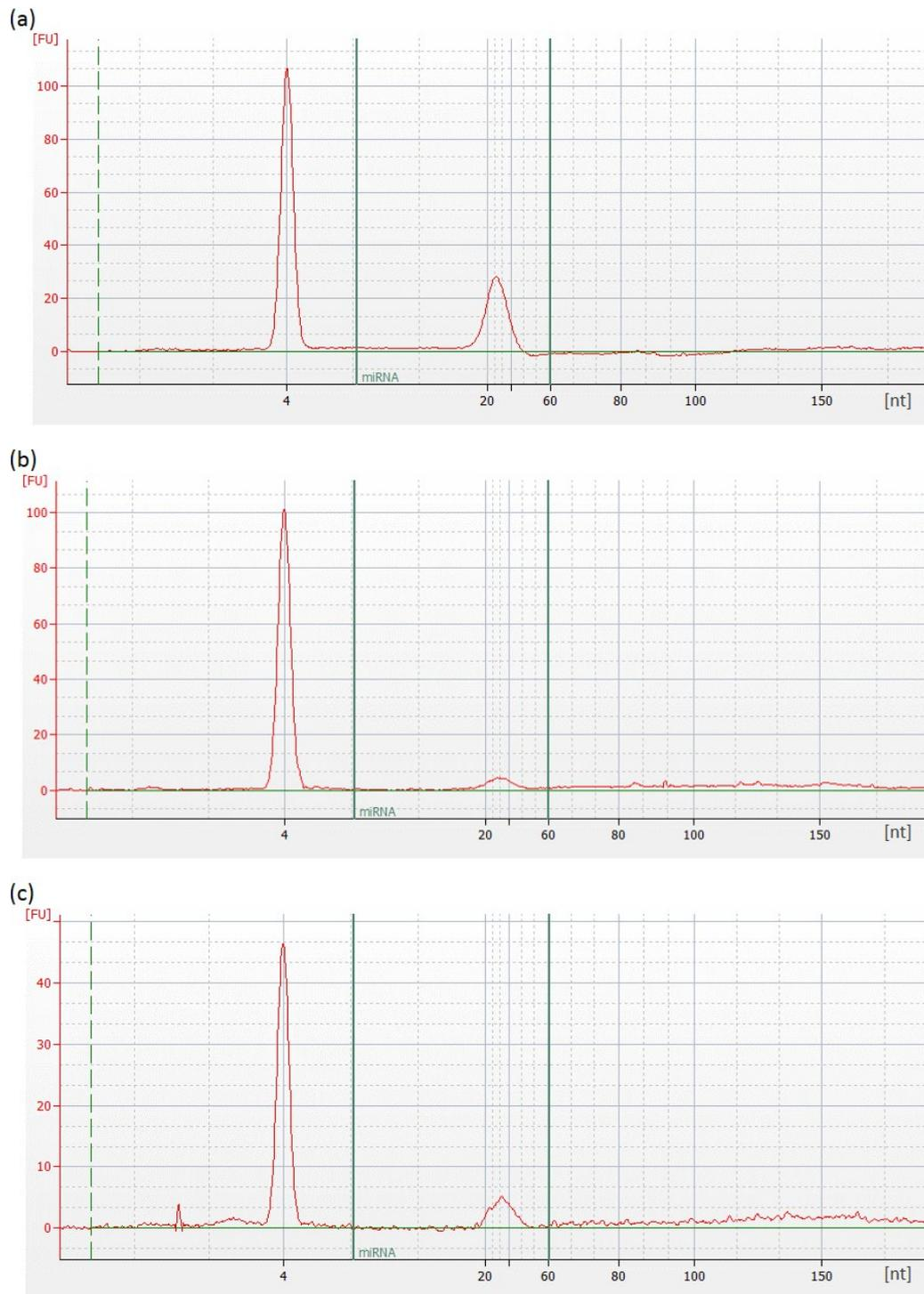
Supplementary Figure S7. Quality control of extracted RNAs. Bioanalyzer analyses of RNAs isolated from (a) the ultracentrifuged pellets from conditioned MDA-MB-231 cell culture medium, (b) EVs captured on magnetic beads, and (c) the supernatant. Most RNAs were within the miRNA range.
