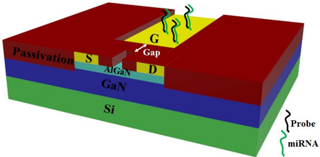
Supplementary Figure S3. Schematic illustration of AlGaN/GaN HEMT sensor capturing target miRNA using specific probes immobilized on the gate electrode.
