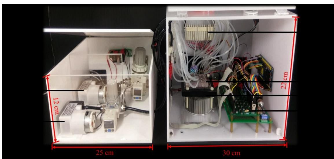
Supplementary Figure S2. Photographs of the home-made portable control device, which was composed of (a) a positive pressure source (compressor), (b) a negative gauge pressure source (vacuum pump), (c) electromagnetic valves (EMVs), (d) a microfluidic chip, (e) a TE cooler (thermal control module), and (f) a control circuit.
