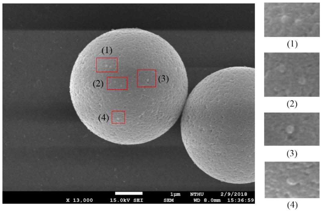
Supplementary Figure S5. The zoomed-in SEM images of captured EVs on the surface of magnetic beads showed that the morphology of captured EVs were still intact and sphere-like.
