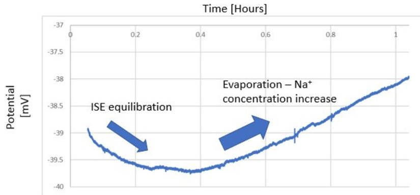
**Figure S5-** Changes in the response of a stand-alone Na<sup>+</sup> ISE (which did not include the microfluidics module) exposed to a 0.01M NaCl solution over a one-hour period.
