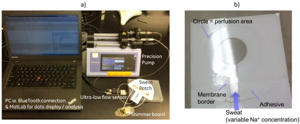
**Figure S4- a)** Lab based sweat testing system with notebook, syringe pump and flow sensor. **b)** Skin mimicking interface using permeable membrane and microfluidics channel for sweat or salt solution delivery
