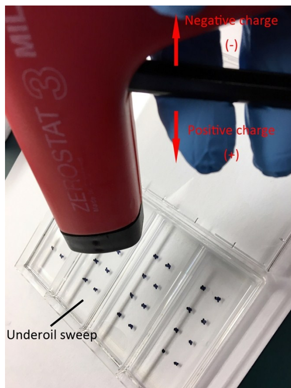
Fig. S8. Electrostatic perturbation applied via anti-static gun to accelerate underoil sweep patterning. The gun was held about 5 cm above the oil-air interface while positive and negative charges were alternatively applied to the oil layer. The oil layer vibrated during this process, which adds momentum to the aqueous drop under oil and thus help it to penetrate the thin layer of oil underneath. Typically, the momentum from one positive and negative cycle is enough to trigger a complete replacement of oil by aqueous media.
