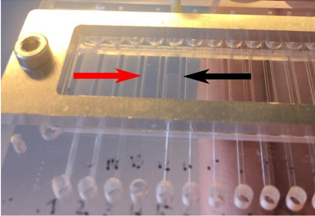
**S.Fig 2** Photo of the interfaces between water and air (black arrow), and water and oil (red arrow) in the fluidic channels.
