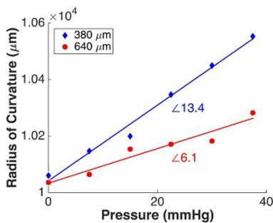
**Supplementary Figure 3** Hemispherical pressure vessel characterization. Blue diamonds and red circles represent data for 380 and 640 μm thick pressure vessels, respectively. The thickness of the pressure vessel was controlled using different volumes of PDMS.
