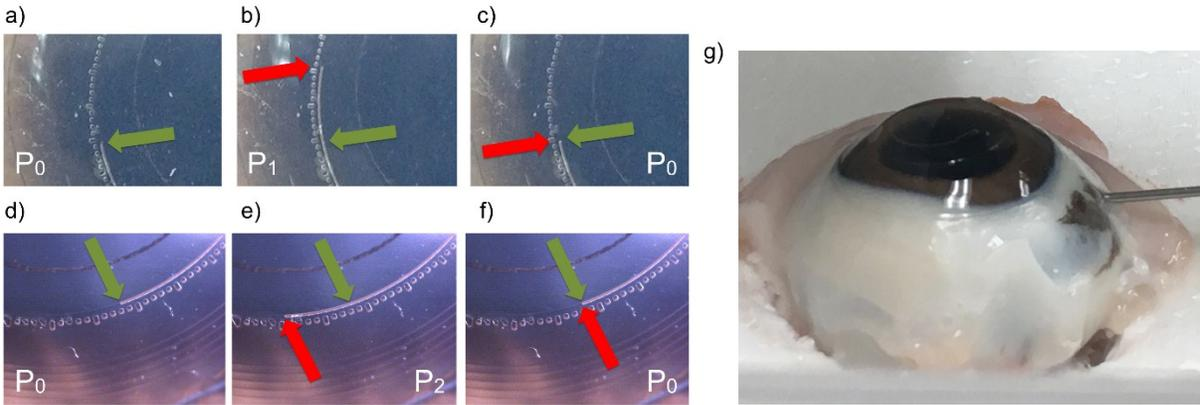
**Supplementary Figure 5** a-f) Pictures of the MSS-CL on a porcine eye. a-c) The pictures taken by a smart-phone camera. d-f) The pictures taken by a stereomicroscope.  $P_0$ ,  $P_1$ , and  $P_2$  correspond to 7, 34, and 22 mmHg, respectively. g) The picture of a porcine eye experiment setup. MSS-CL was placed on the porcine eye and it was pressurized using a 16 Ga needle attached to the Elveflow OB1 pressure generator.
