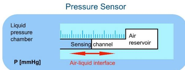
**Supplementary Figure 1** Pressure sensor operation principle based on Boyle's law. As the pressure increases (decreases) inside the liquid pressure chamber the air-liquid interface moves toward the air (liquid) reservoir in order to keep the pressure and volume product constant.
