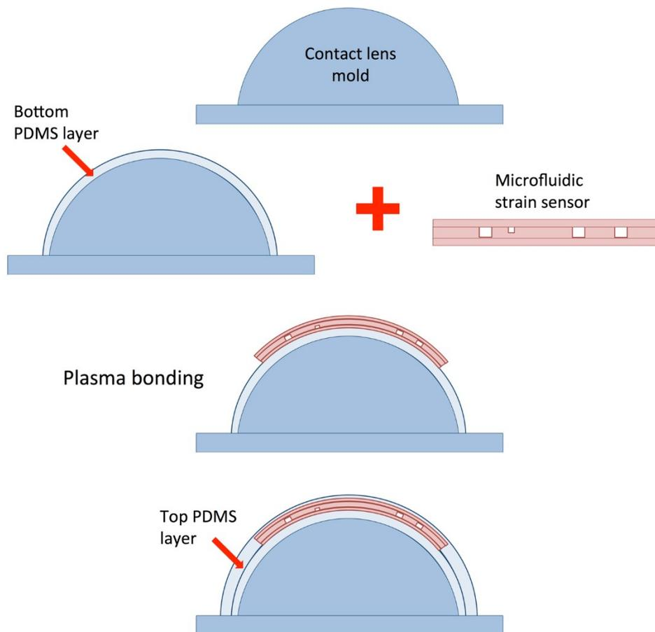
**Supplementary Figure 4** Fabrication protocol of the MSS-CL. First, a contact lens mold was covered with a thin PDMS layer in order to obtain the bottom PDMS layer of the MSS-CL. Then, the microfluidic strain sensor was bonded to this thin PDMS layer. The standard plasma-bonding techniques were applied. Finally, this combined structure was covered with a thin PDMS layer.
