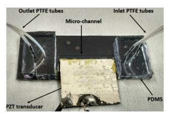
**Supplementary Figure 2:** Photograph of the experimental set-up
