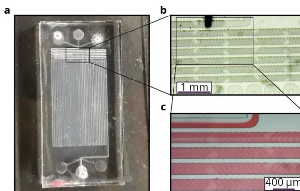
**Figure S3 – PDMS microfluidic device with staggered herringbone mixer.** Photograph of PDMS microfluidic device (a), a zoom in on the staggered herringbone mixer at the start of the device (b) and the mixing using water and a red dye (c).
