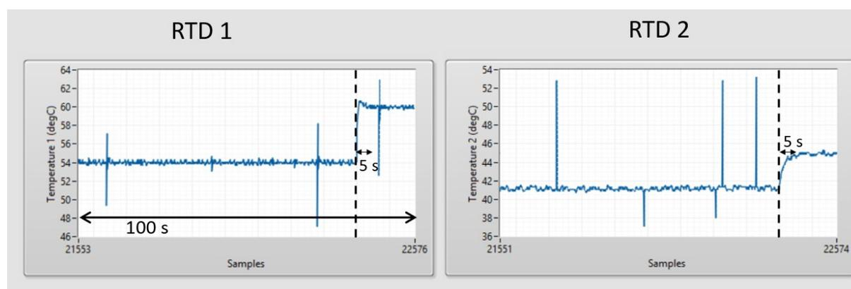
**Fig S1 – illustration of the stability of the temperature control over time.** The temperature is very stable over time as illustrated here over the first 80 seconds of the figure, and the response when the target temperature is modified is very quick at both RTD positions (typically 5 seconds, as illustrated). The noise peaks/spikes are probably caused by interference with the RTD by the pulse-width modulated (PWM) square wave signal that is used to switch the heaters on/off.
