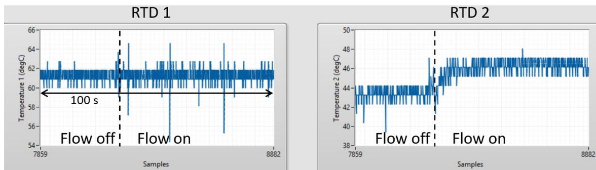
**Fig S2 – illustration of the stability of the temperature control over time with respect to flow off and flow on conditions.** The temperature at the downstream measurement position (RTD 2), raises with 2 to 3 °C, when the flow is switched on. The regulated temperature at RTD 1, does not vary with flowrate. The noise peaks/spikes are probably caused by interference with the RTD by the pulse-width modulated (PWM) square wave signal that is used to switch the heaters on/off.
