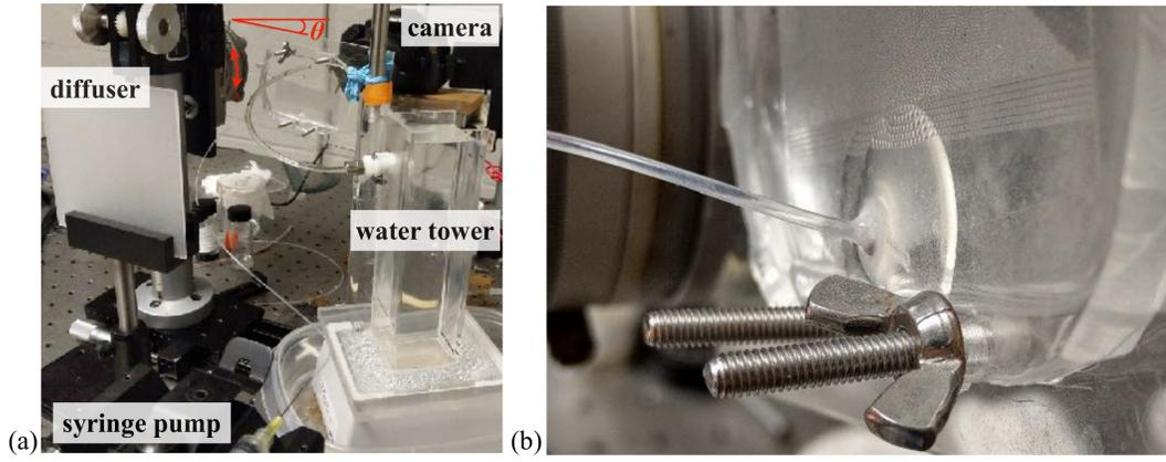
FIG. 1. (a) Photo of the full setup (light source excluded), with an apparent positive channel angle  $\theta$ . (b) Close up photo of the inlet at the bottom of the experiment, where the tubing was set with a downward angle and was covered of extra PDMS to prevent any leakage.
