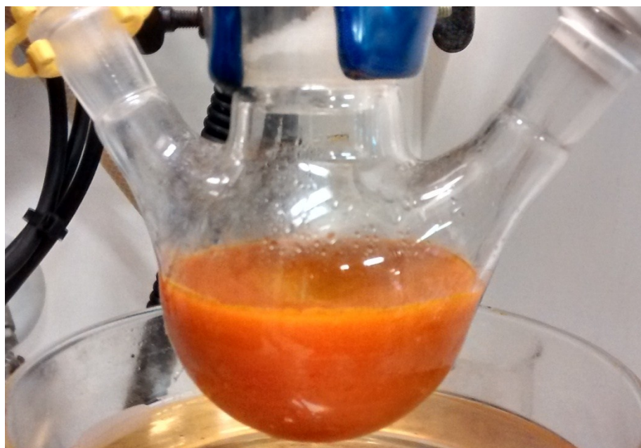
Figure S1 | Crude product. Reaction vessel showing the bright orange product right before filtering it off.
