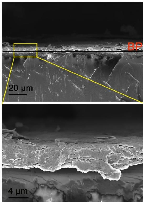
**Fig.S9** The cross-section SEM image of the electrode.
