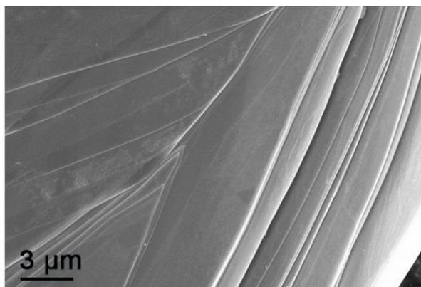
**Fig. S1** SEM image of bulk BP crystal.
