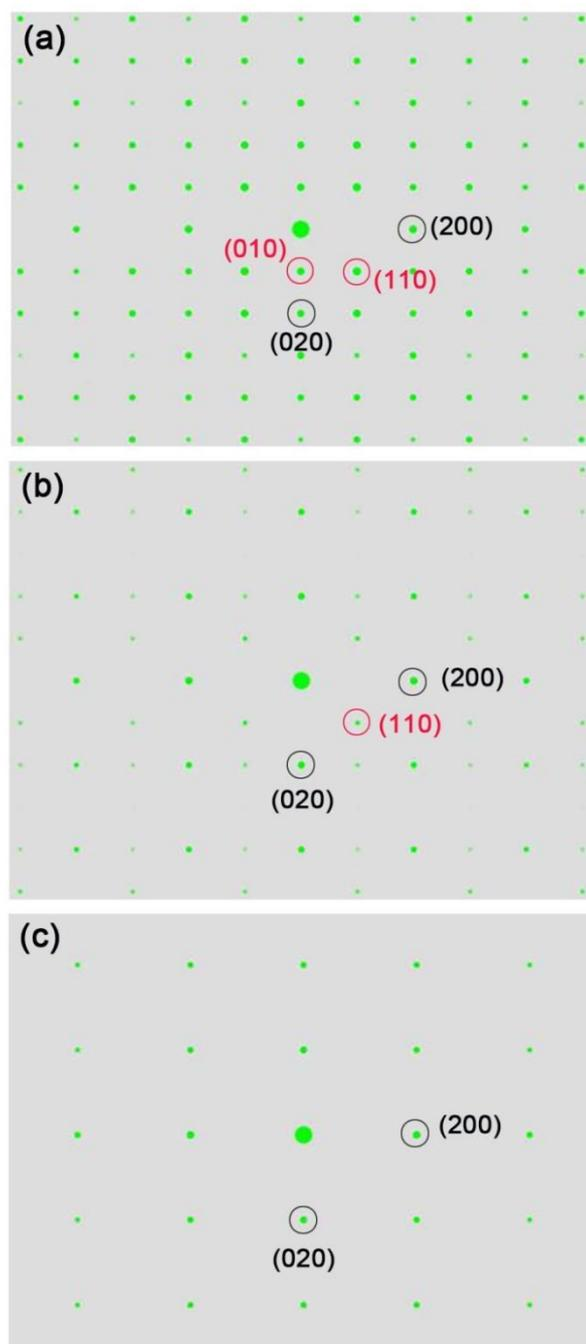
**Fig. S8** Simulated SAED patterns: (a) Single-layer, (b) Two-layer, and (c) Multi-layer BP. The BP crystal structure from reference<sup>1</sup> is used and simulated using CrystalMaker Software LTD.
