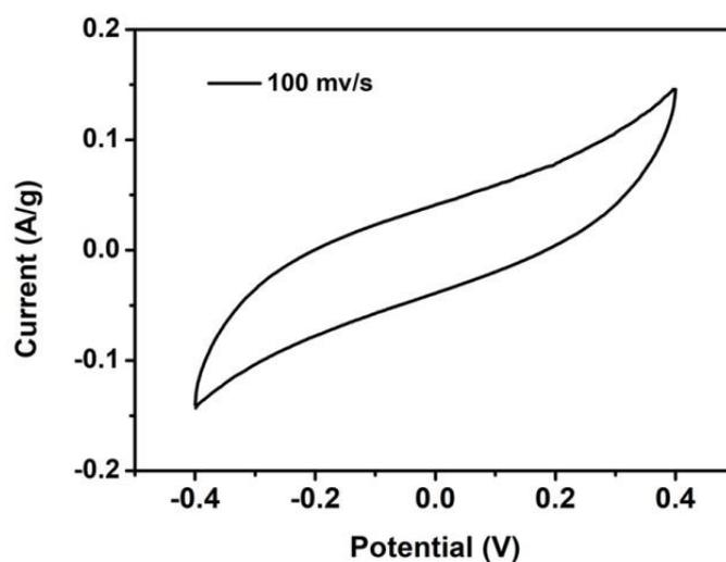
**Fig. S10** Cyclic voltammogram of all-solid-state supercapacitor with bulk BP as the electrode materials acquired at a scanning rate of 100 mV/s.
