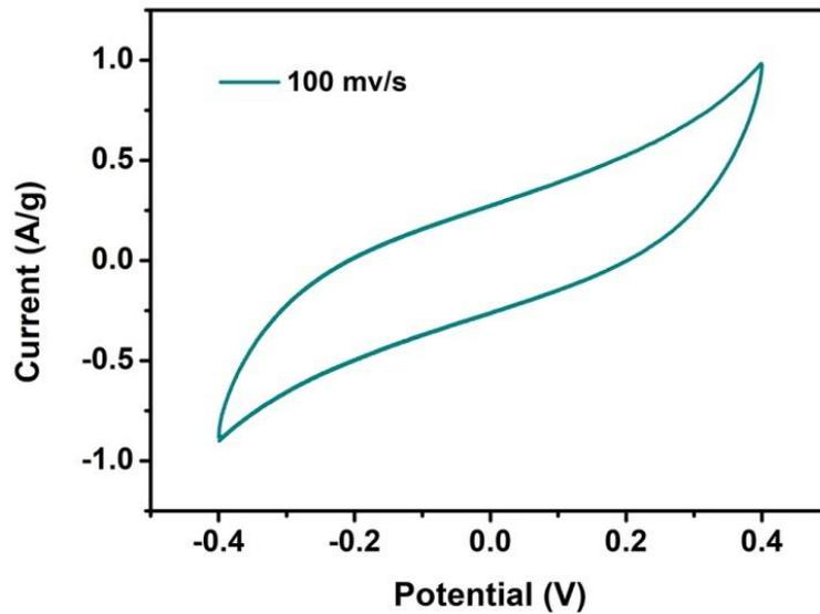
**Fig. S11** Cyclic voltammogram of the all-solid-state supercapacitor composed of BP nanosheets as the electrode materials obtained at a scanning rate of 100 mV/s.
