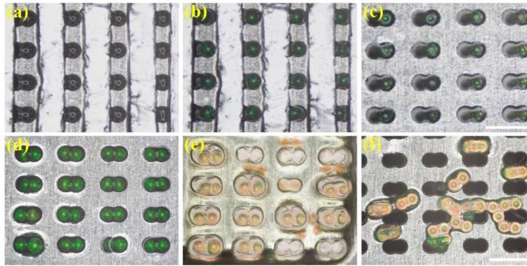
**Figure S4.** (a-f) The real images of the generation process of the photonic barcodes in the double-hole negative mold. The scale bars are 1mm.
