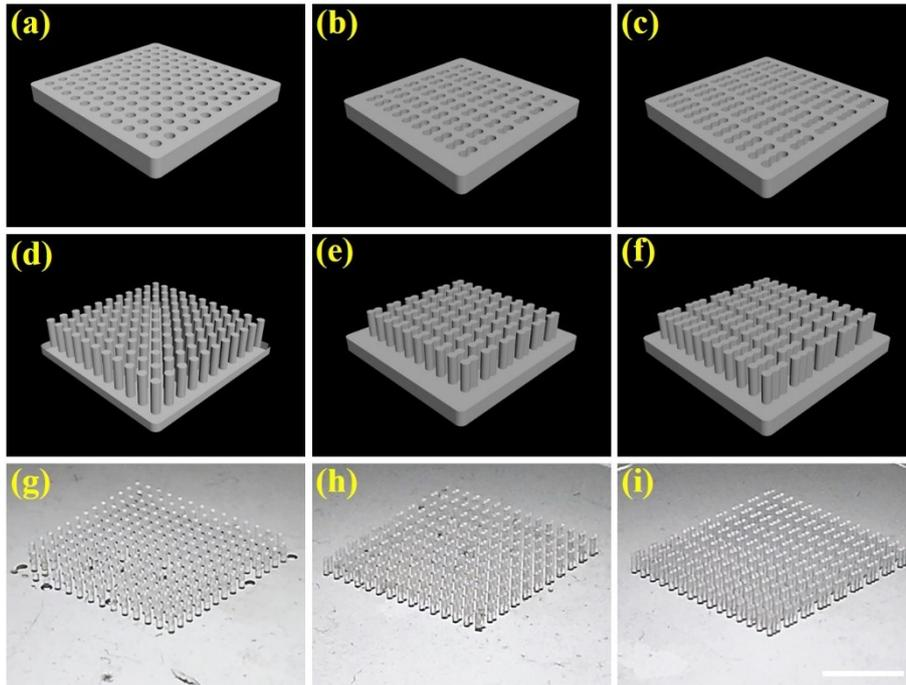
**Figure S1.** (a-c) The stereo illustrations of the negative molds with different hole arrays; (d-f) the stereo illustration of the positive molds with different cylindrical arrays; (g-i) the images of the real PDMS positive molds. The scale bar is 0.5cm.
