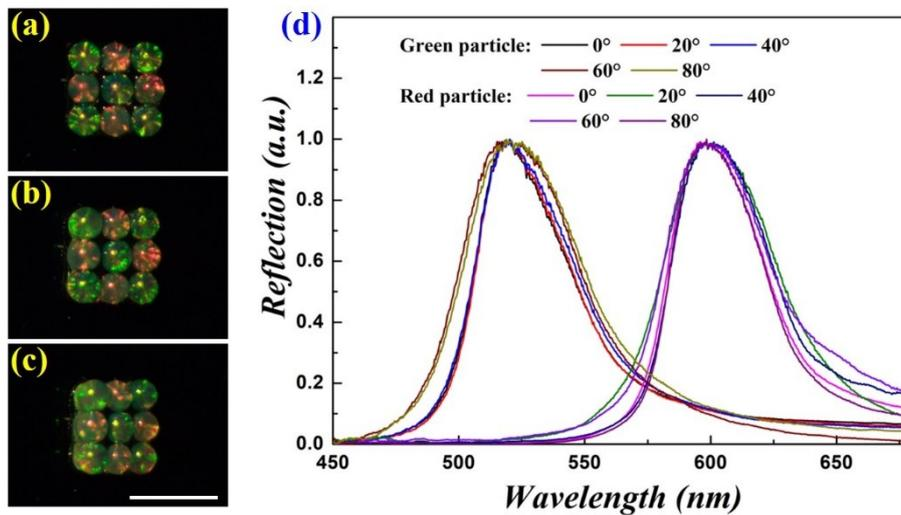
**Figure S5.** (a-c) The optical image characterizations about the angle-independent property of the photonic barcodes. The observing angles (angle between the horizontal plane and the  $3 \times 3$  barcode) are  $0^\circ$ ,  $20^\circ$  and  $40^\circ$  in
