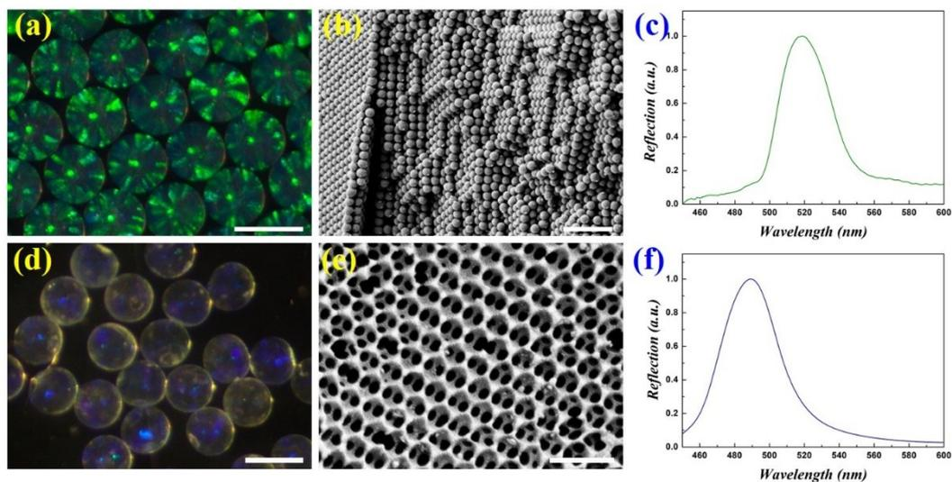
**Figure S6.** (a-b) The optical (a), microstructures (b) and spectral (c) images of the PhC microparticles; (d-f) the optical (d), microstructures (e) and spectral (f) images of the egg white inverse opal particles. The scale bars are 300  $\mu\text{m}$  in (a, d), 1  $\mu\text{m}$  in (b) and 500 nm in (e).
